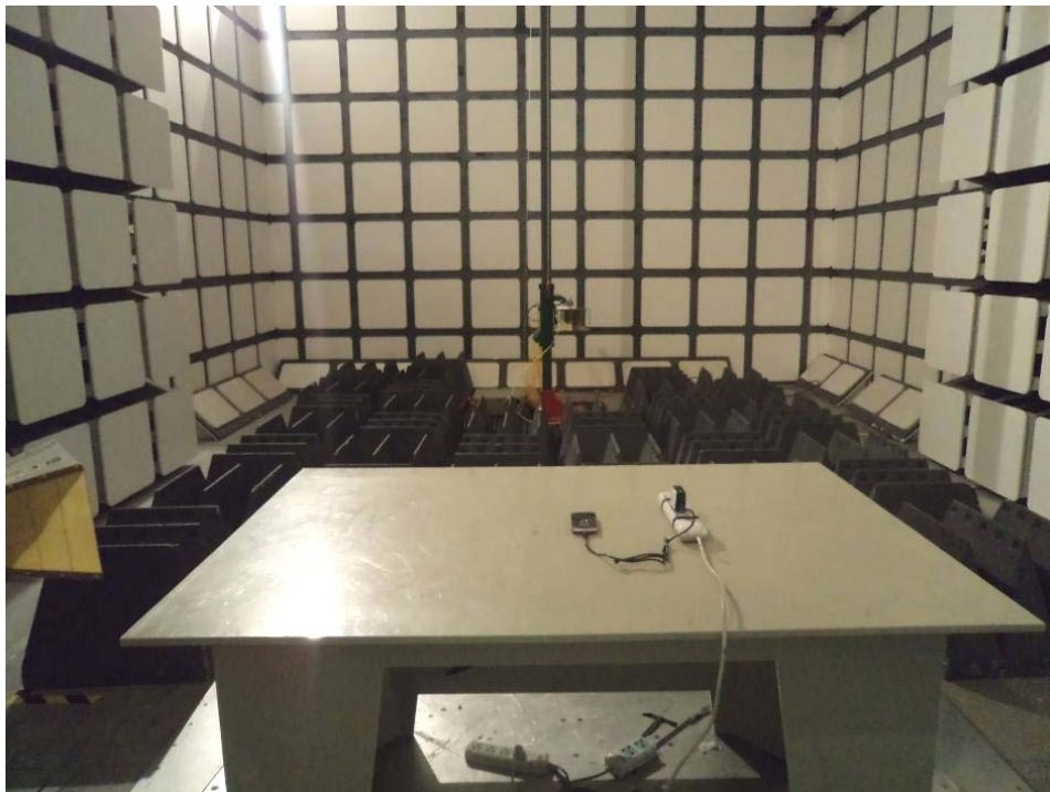
Above 1 GHz: Radiated Emissions - Rear View
