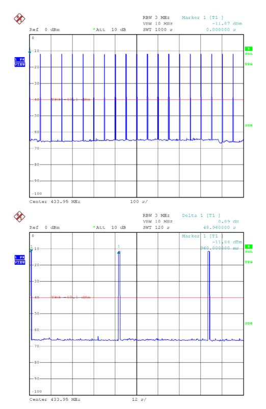
Timing Plot – Pursuant to FCC Part 15 Section 15. 231(e) Requirement (Pass/Fail)
