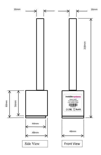
The label is self-adhesive, the Model No and ID's will be affixed to the front face of the Tx housing
