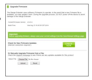
Manual Firmware Upgrade: In the case that the Range Extender does not have access to the Internet, you can manually upgrade the firmware by downloading the firmware file from the Amped Wireless Elite Support website. The firmware update is downloaded as a zip file and you will need to have an unzipping program to open the file. Inside the file will be a text document with details on the current firmware release and instructions on how to upgrade the firmware.
