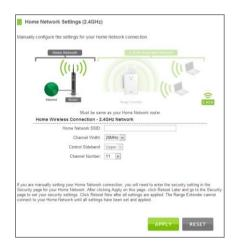
Channel Width: Wi-Fi operates in two separate channel widths, 20Hz and 40Hz. 20Hz allows operation on channels 1-11, while 40Hz is 5-11. 40Hz allows for faster speeds. Select the channel width you wish to use for your network. This setting must match that of your Home Network for a successful connection.
