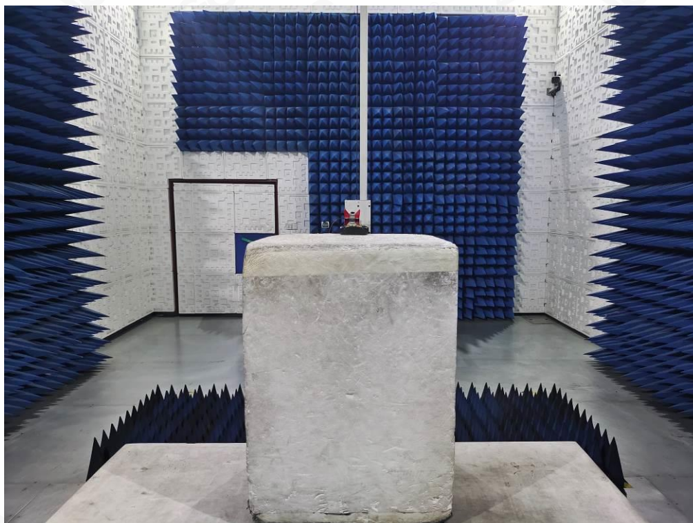
FCC RADIATED EMISSION TEST SETUP ABOVE 1GHZ
