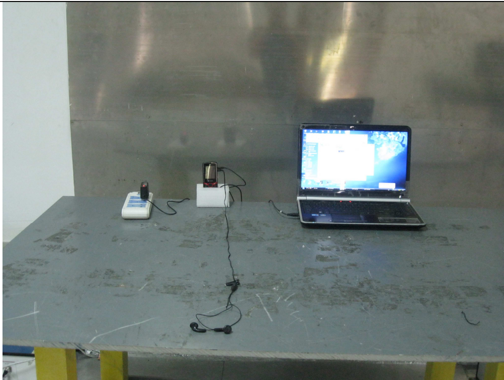
Conducted Emissions Test Setup Front View
