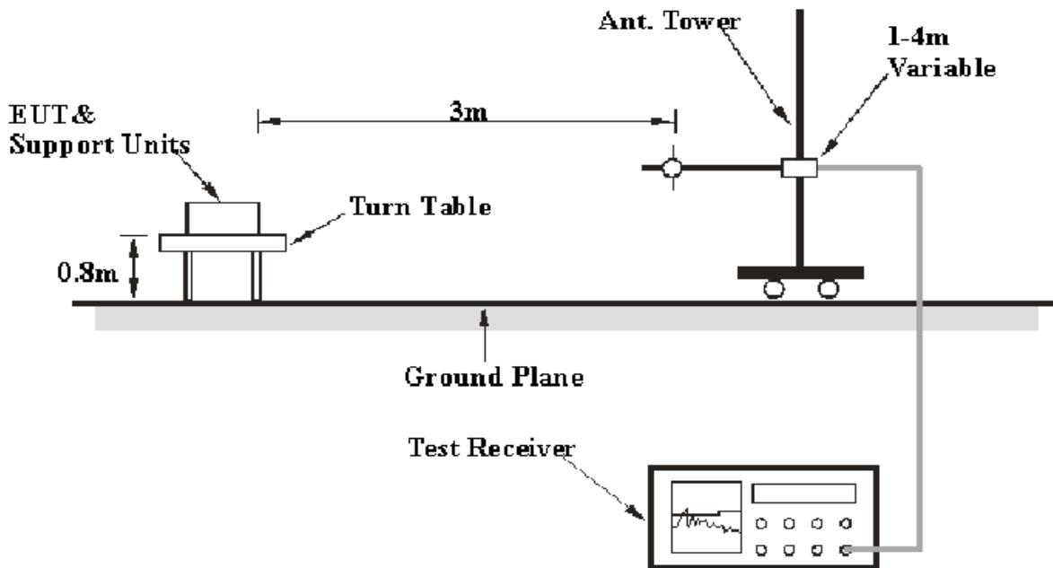
The radiated emission tests were performed in the 3 meters chamber B test site, using the setup accordance with the ANSI C63.4-2009. The specification used was the FCC Part 15.109 Class B limits.
