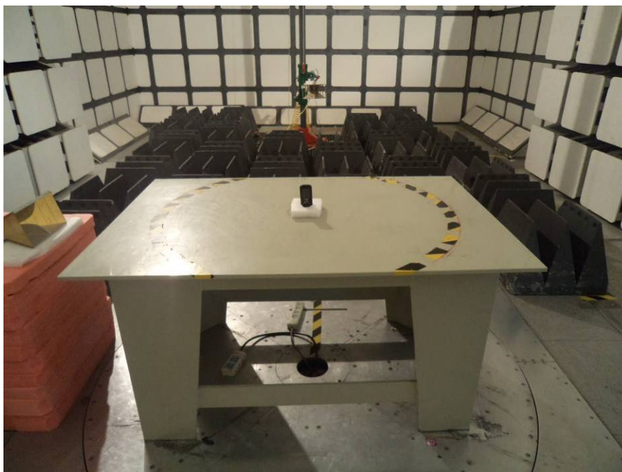
Radiated Emissions View (1-25 GHz)
