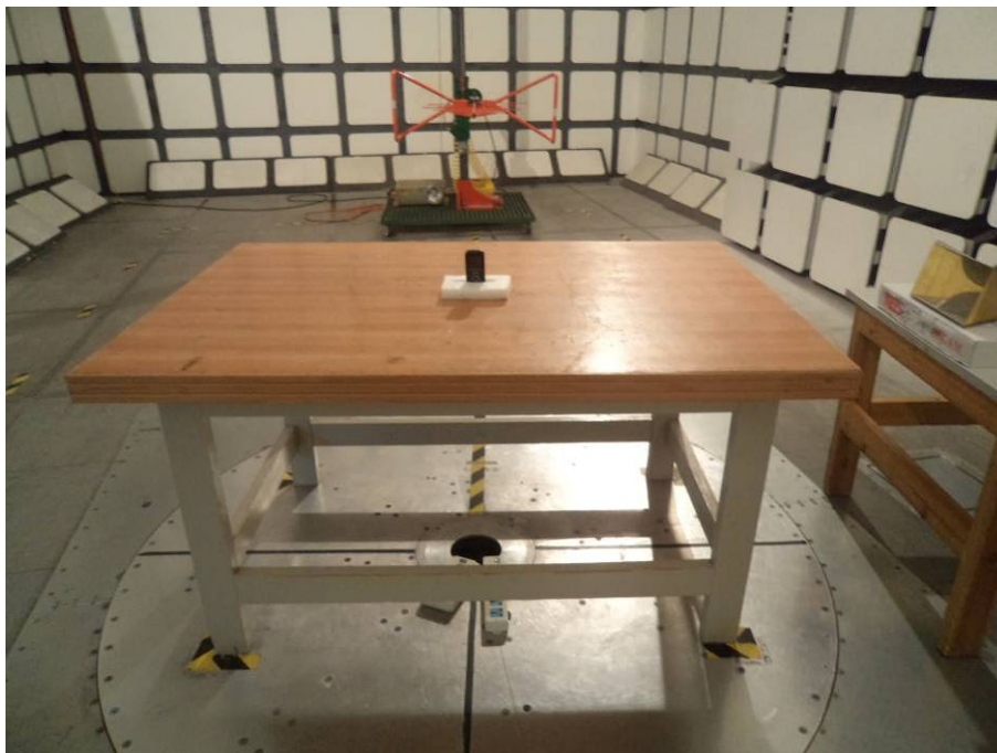
Radiated Emissions View (30-1000 MHz)
