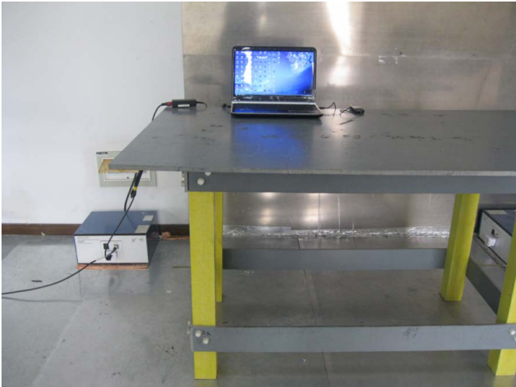
Conducted Emissions Test Setup - Front View
