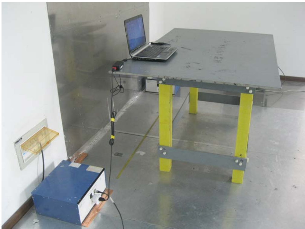
Conducted Emissions Test Setup - Side View
