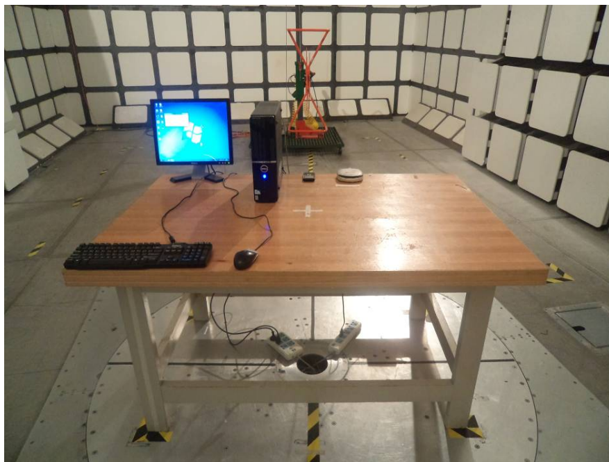
Radiated Emissions – Rear View (downloading mode, 30-1000 MHz)
