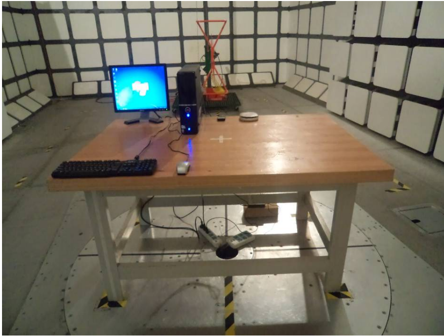
Radiated Emissions-Front View
