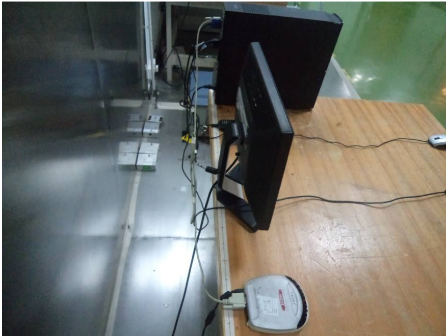
Conducted Emissions - Side View (downloading mode)
