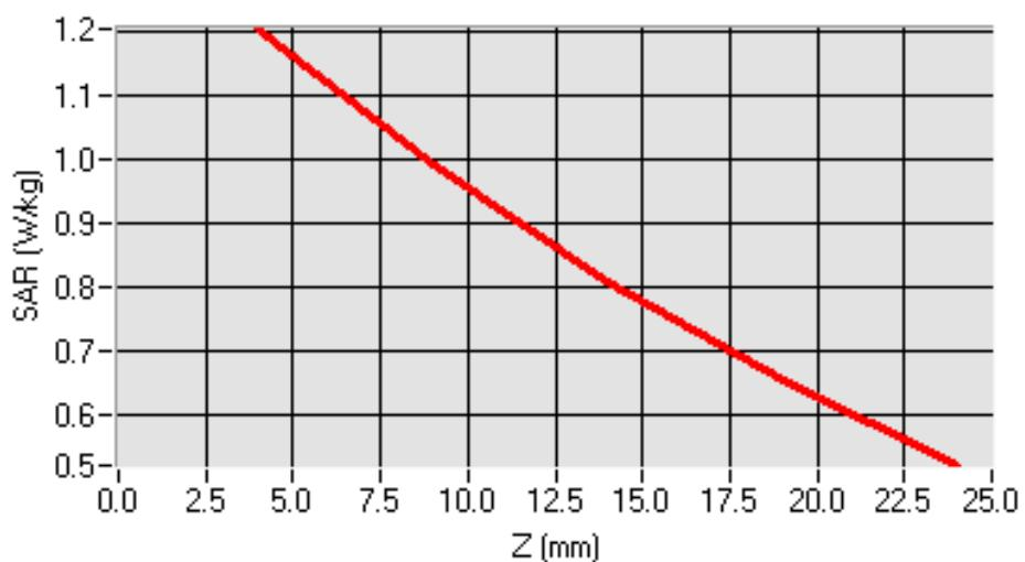
Test mode: GSM850, middle channel (Right Head Cheek)
