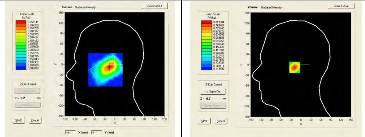
**SAR, Z Axis Scan (X = -15, Y = -8)**
