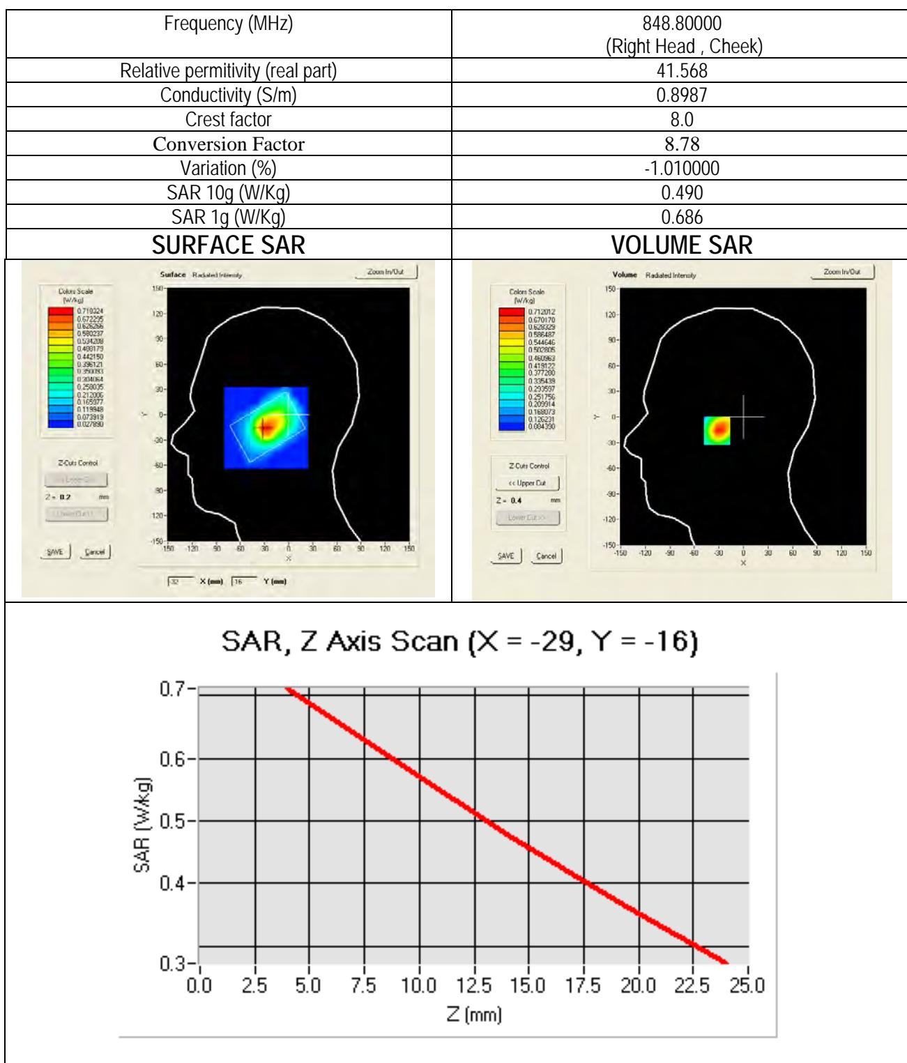
Test mode: GSM850, low channel (Right Head Tilt)
