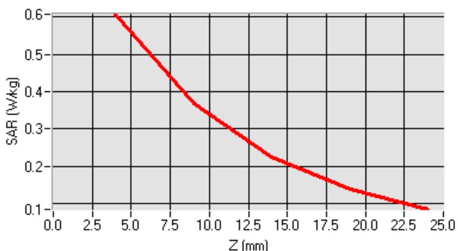
Test mode: GSM1900, high channel (Left Head Cheek)
