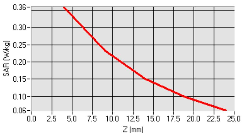
Test mode: GPRS1900, high channel (Body LCD-DOWN)
