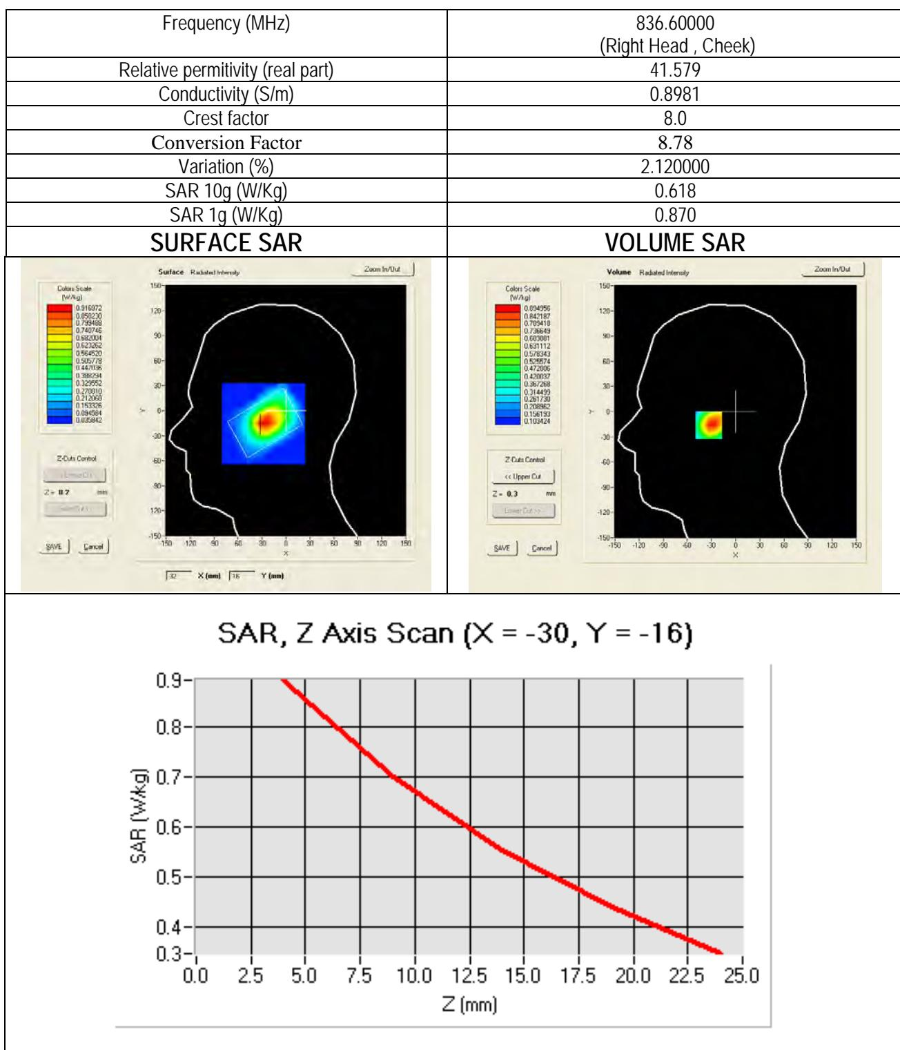
Test mode: GSM850, high channel (Right Head Cheek)
