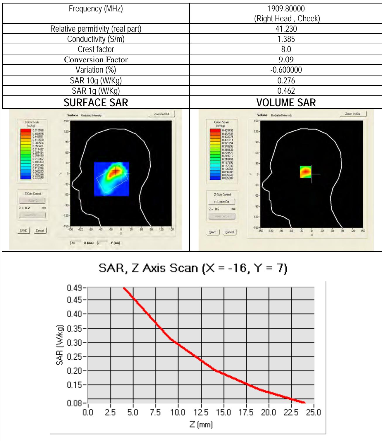
Test mode: GSM1900, high channel (Right Head Tilt)
