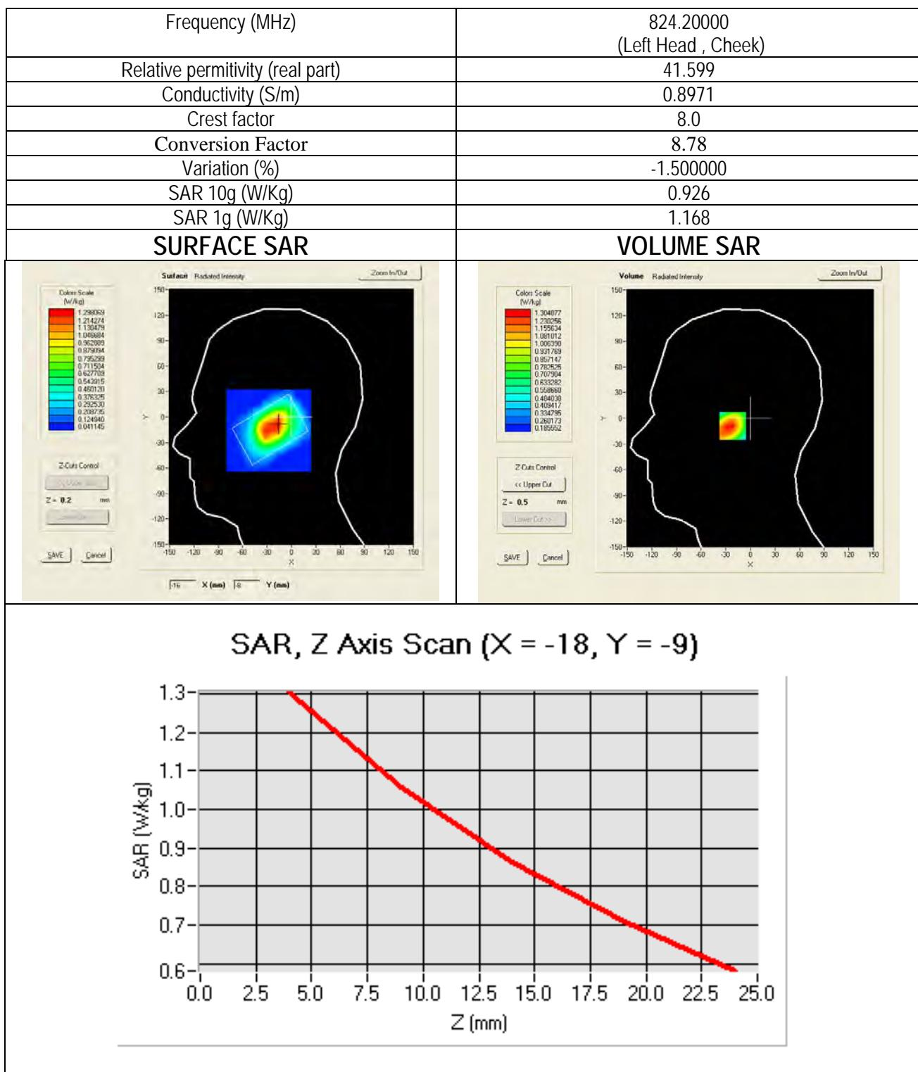
Test mode: GSM850, middle channel (Left Head Cheek)
