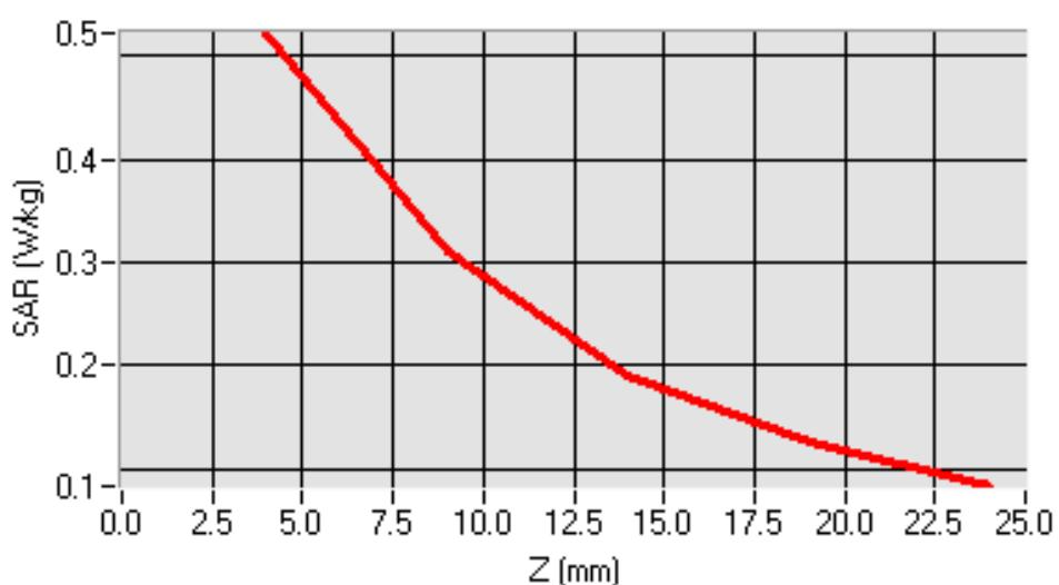
Test mode: GSM1900, high channel (Left Head Tilt)
