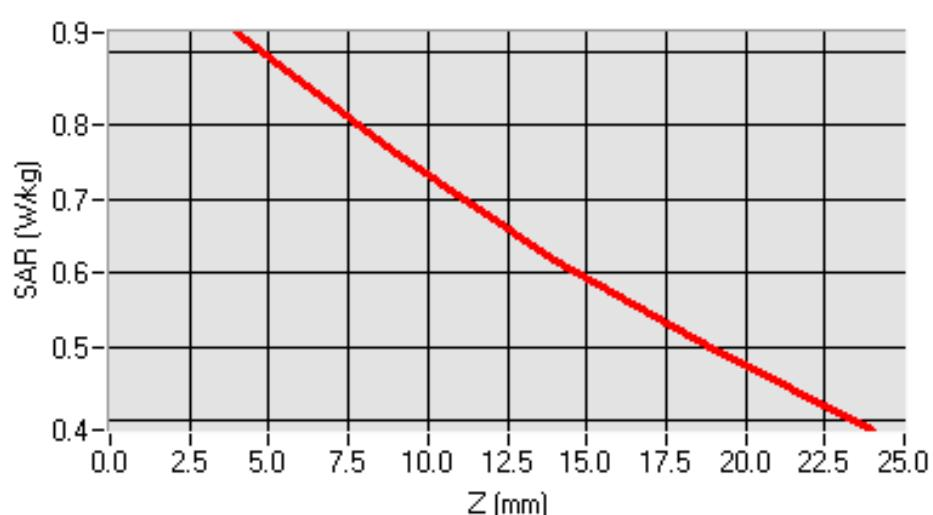
Test mode: GPRS850, high channel (Body-LCD DOWN)
