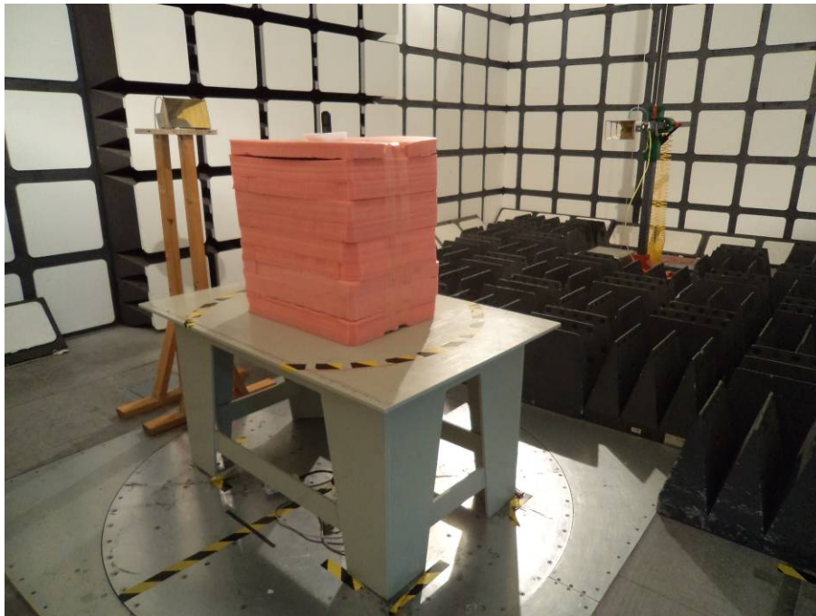
Radiated Emissions Test View (Above 1 GHz)
