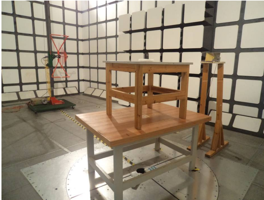
Radiated Emissions Test View (30 MHz-1 GHz)
