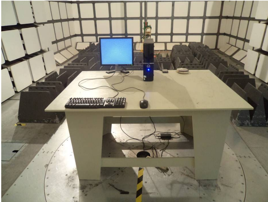
Radiated Emissions – Front View (Above 1 GHz)
