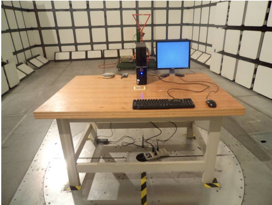
Radiated Emissions – Front View (Below 1 GHz)
