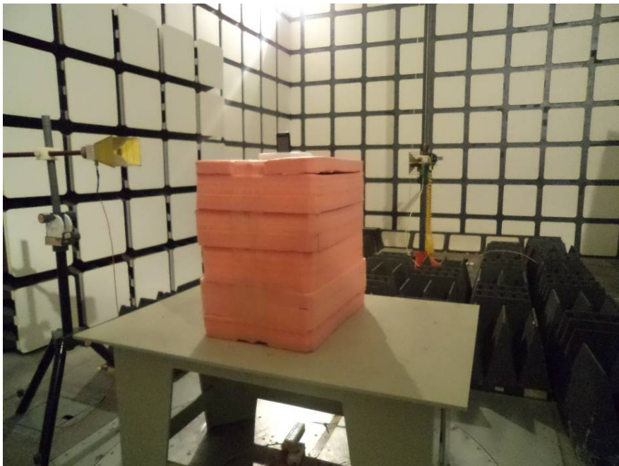
Radiated Emissions Test View (Above 1 GHz)
