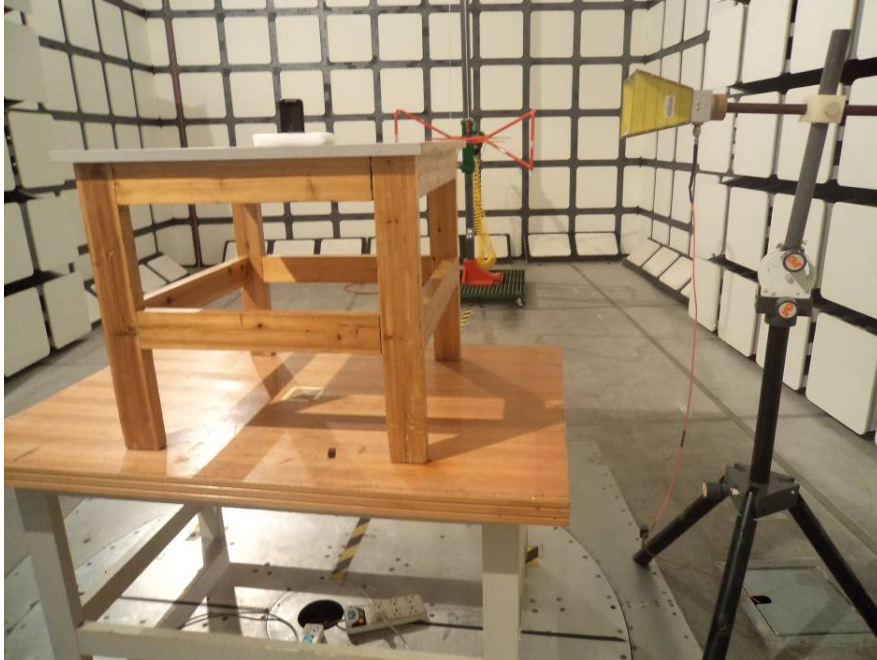
Radiated Emissions Test View (Below 1 GHz)
