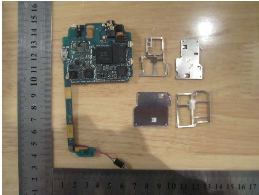
Uncover Without Shielding - Top View
