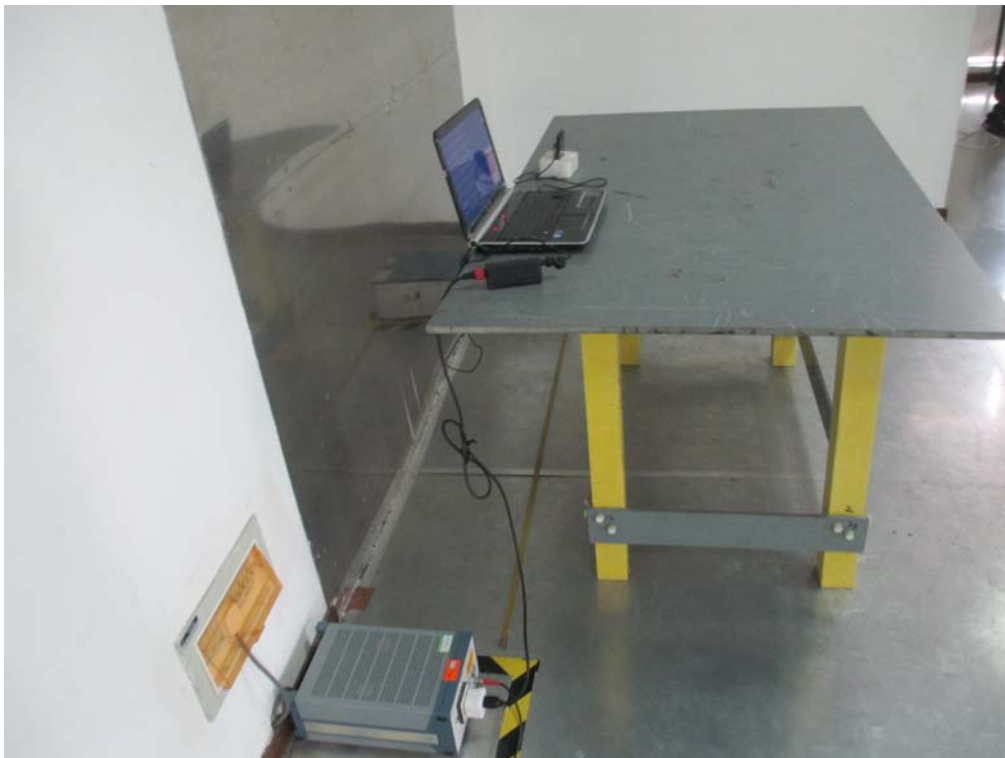
Conducted Emissions Test Setup Side View
