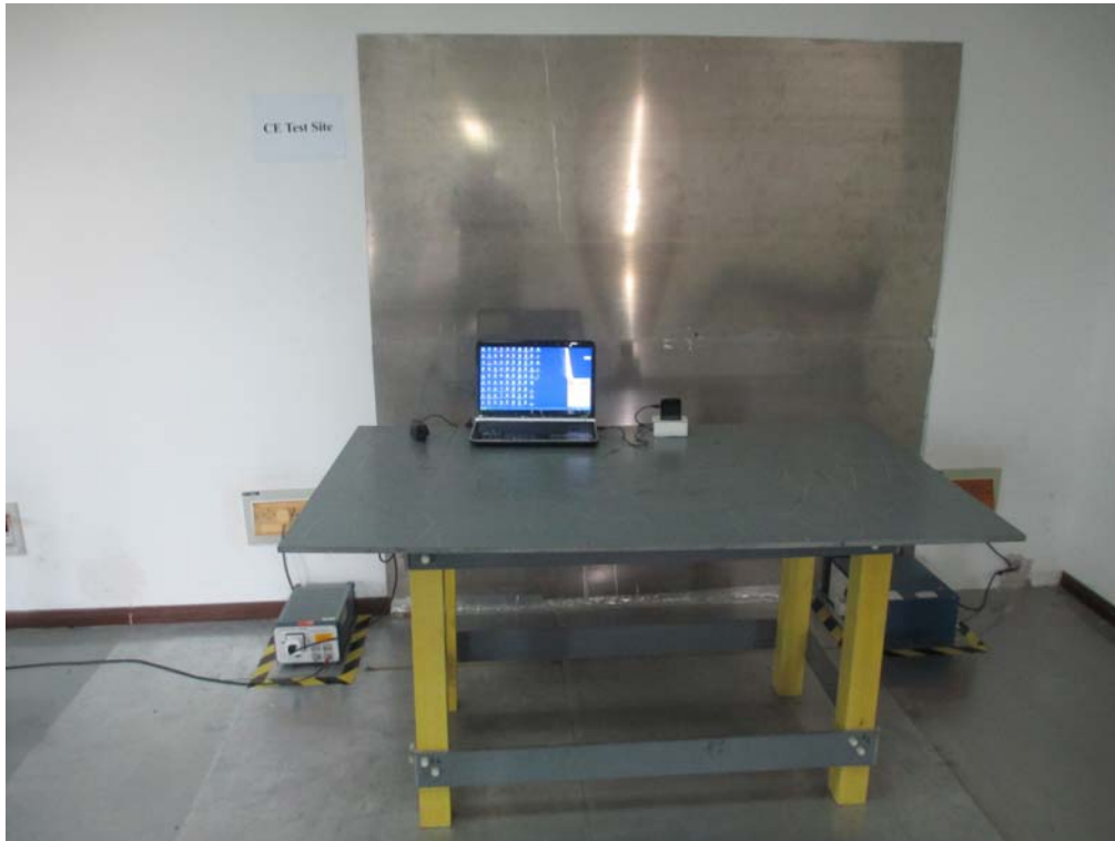
Conducted Emissions Test Setup Front View
