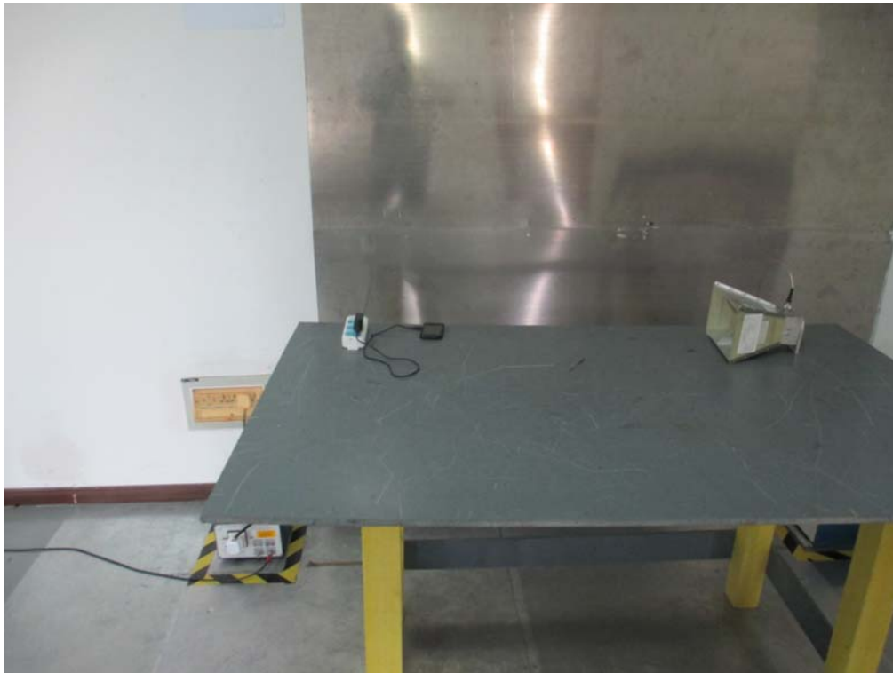
Conducted Emissions Test Setup Front View
