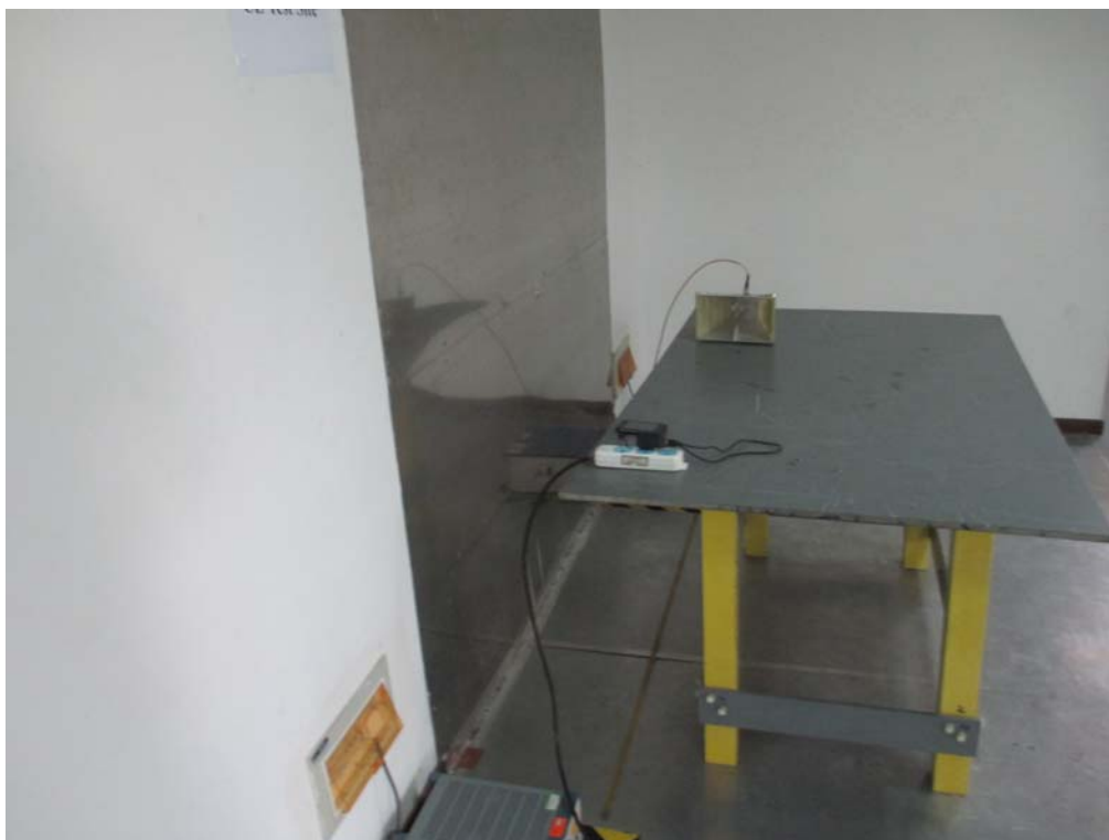
Conducted Emissions Test Setup Side View
