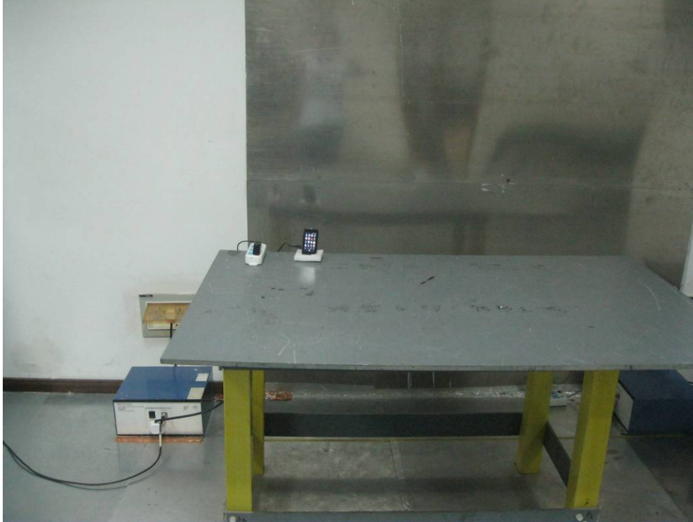
Conducted Emissions Test Setup (GPS receiving) - Front View
