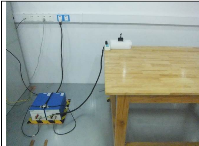
Conducted Emissions Test Setup Front View
