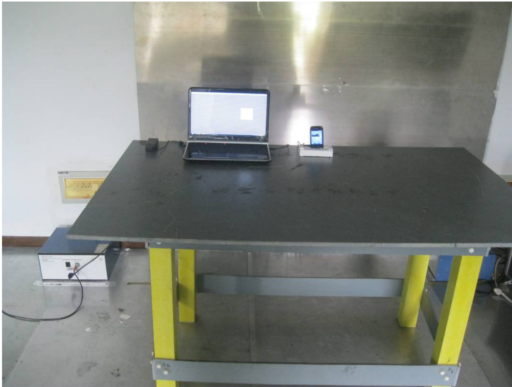
Conducted Emissions Test Setup - Front View
