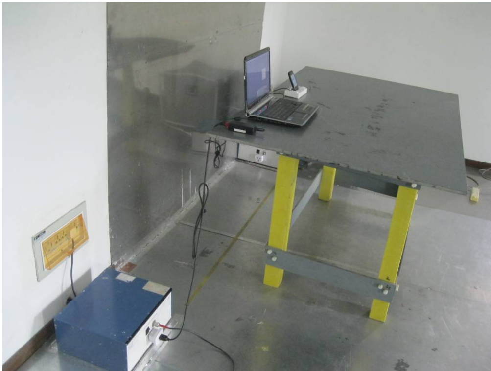
Conducted Emissions Test Setup - Side View
