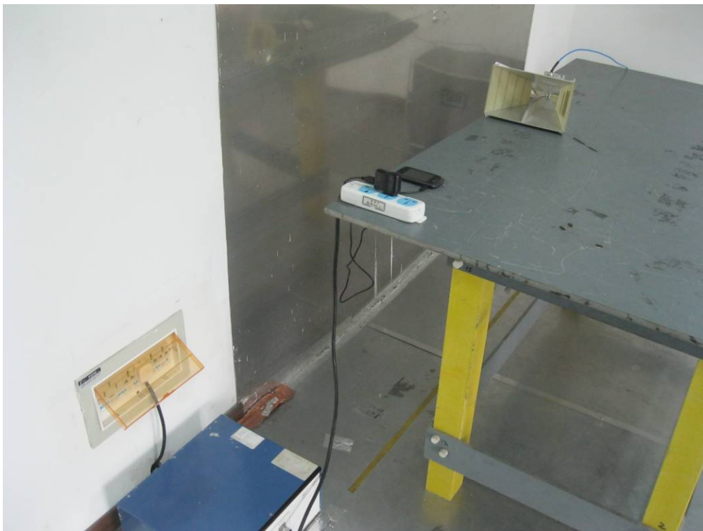
Conducted Emissions Test Setup - Side View
