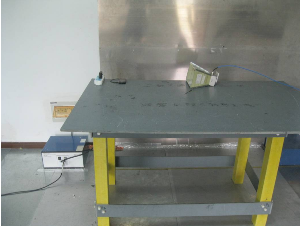
Conducted Emissions Test Setup - Front View
