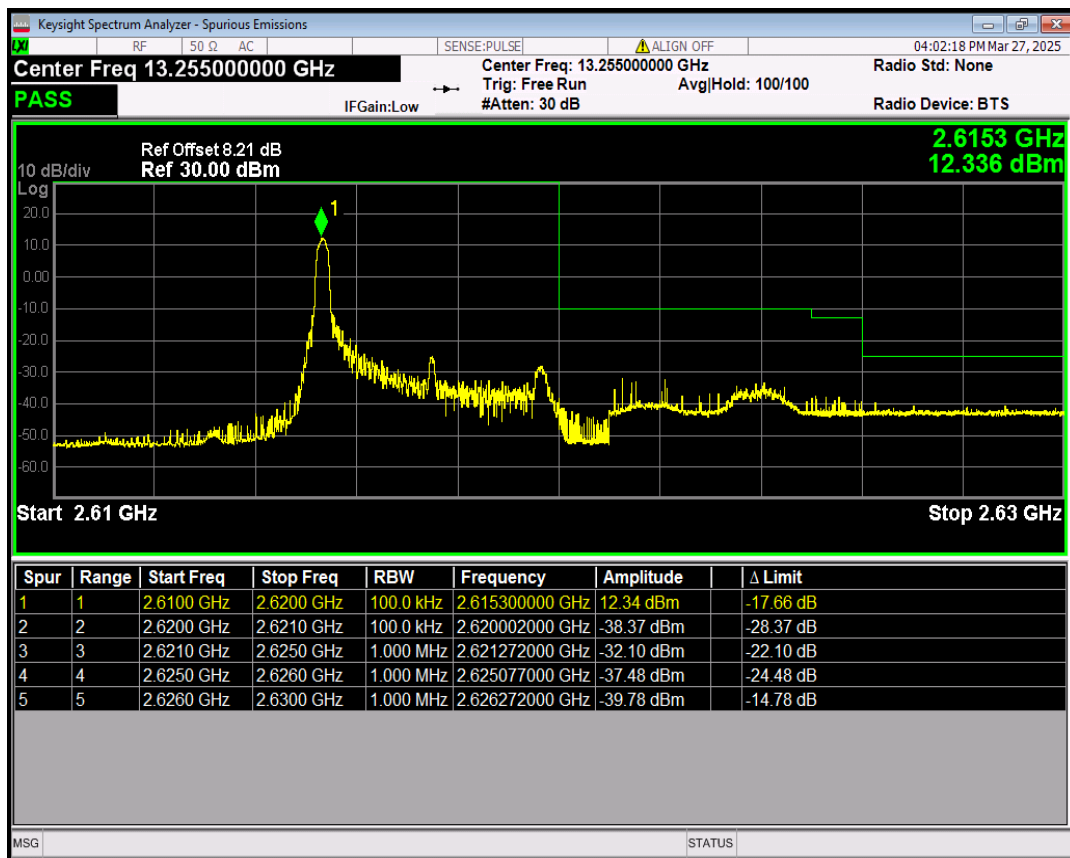
Band38 16QAM BW=5MHz Channel=38225 RB Size=1 Position=#Max
