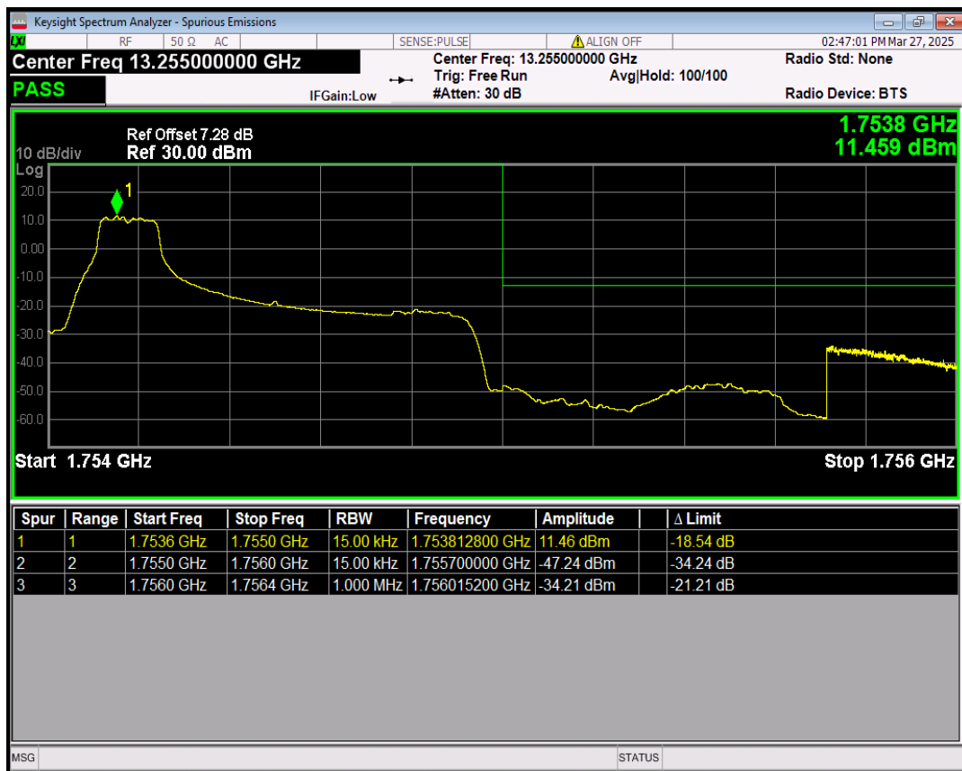
Band4 16QAM BW=1.4MHz Channel=20393 RB Size=1 Position=#Max
