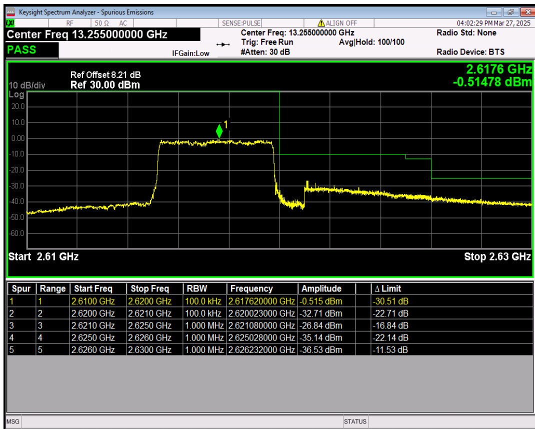
Band38 QPSK BW=10MHz Channel=37800 RB Size=1 Position=#0
