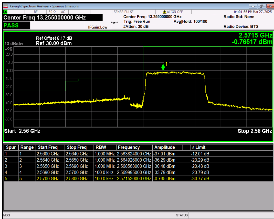
Band38 QPSK BW=5MHz Channel=38225 RB Size=1 Position=#0
