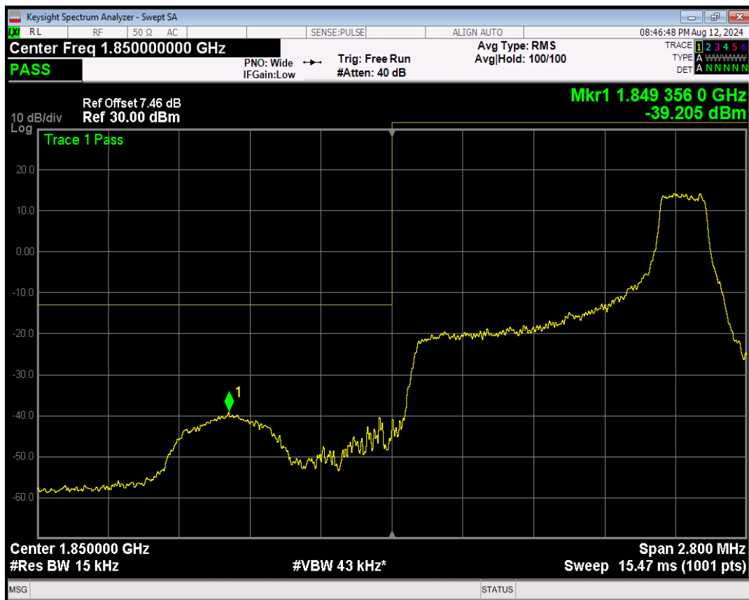
Band2 16QAM BW=1.4MHz Channel=18607 RB Size=6 Position=#0
