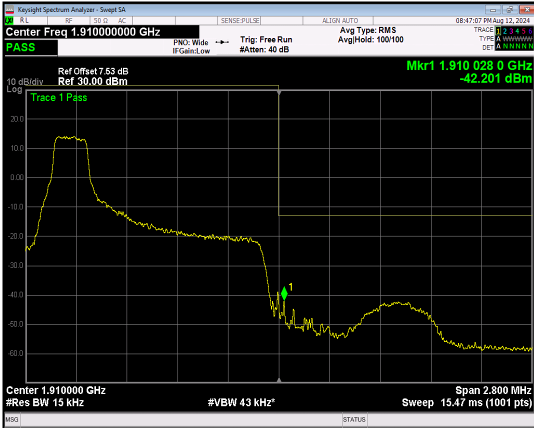
Band2 16QAM BW=1.4MHz Channel=19193 RB Size=1 Position=#Max
