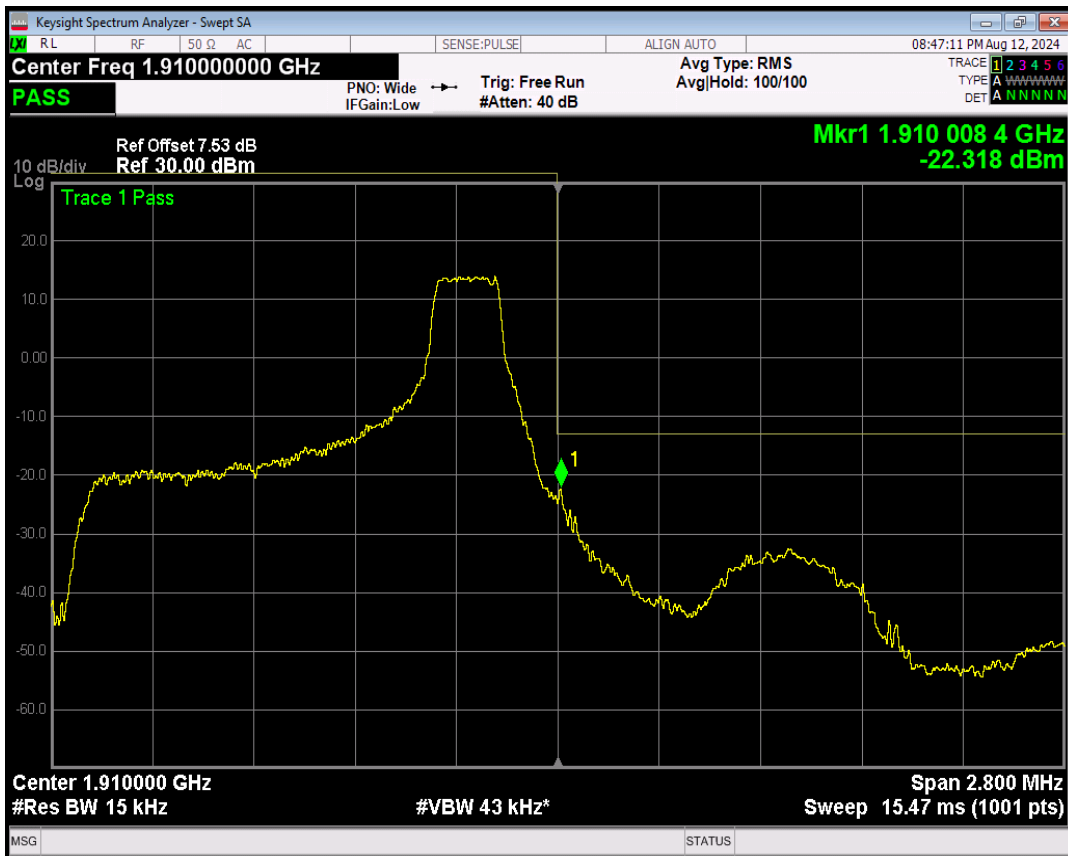
Band2 16QAM BW=1.4MHz Channel=19193 RB Size=6 Position=#0
