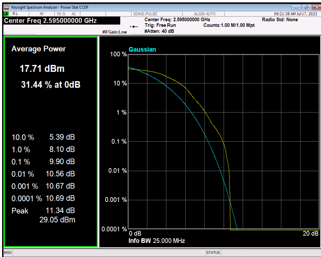
Band38 QPSK BW=15MHz Channel=38000 RB Size=1 Position=#0
