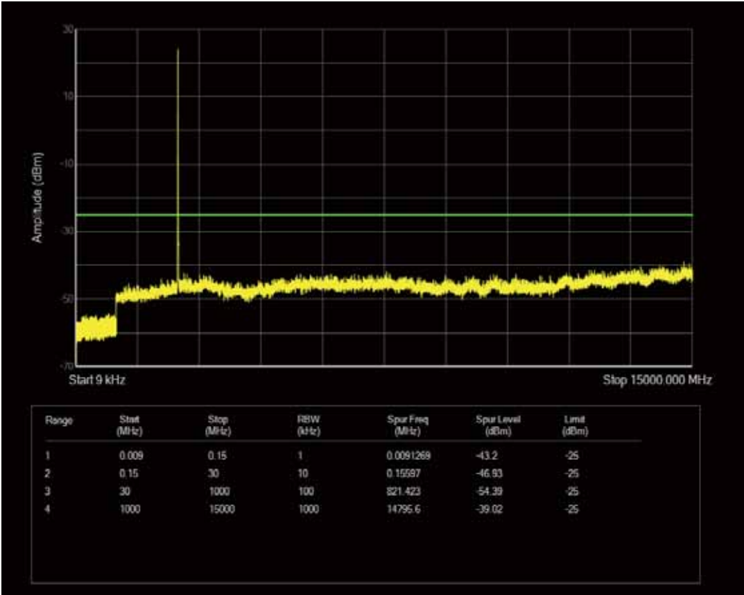
Band7 QAM16 BW=5MHz Channel=20775 RB Size=1 Position=#0
