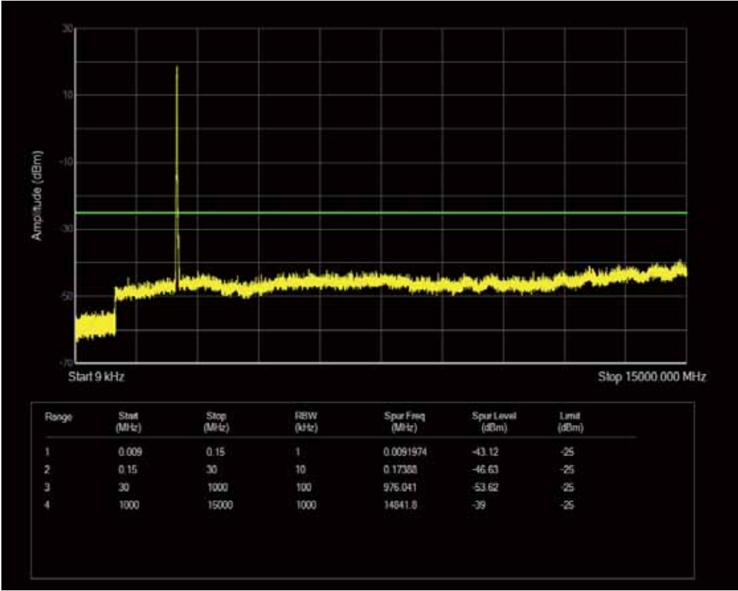
Band7 QPSK BW=20MHz Channel=21100 RB Size=100 Position=#0
