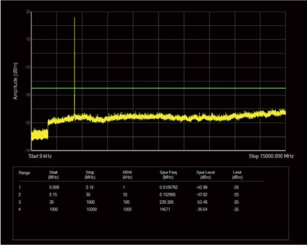
Band7 QPSK BW=10MHz Channel=20800 RB Size=1 Position=#0
