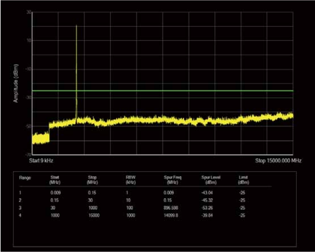
Band7 QPSK BW=15MHz Channel=20825 RB Size=75 Position=#0
