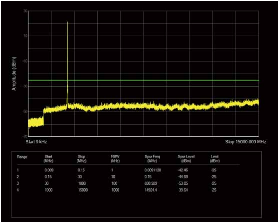
Band7 QAM16 BW=10MHz Channel=21400 RB Size=50 Position=#0
