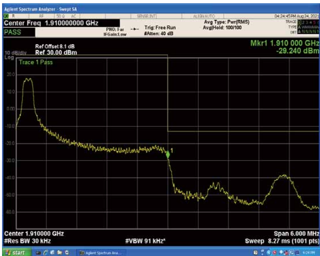
Band2 QAM16 BW=3MHz Channel=19185 RB Size=15 Position=#0
