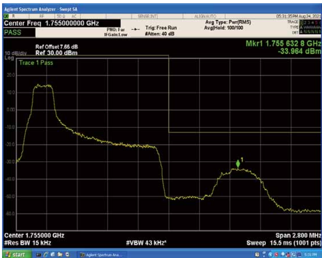
Band4 QAM16 BW=1.4MHz Channel=19957 RB Size=6 Position=#0
