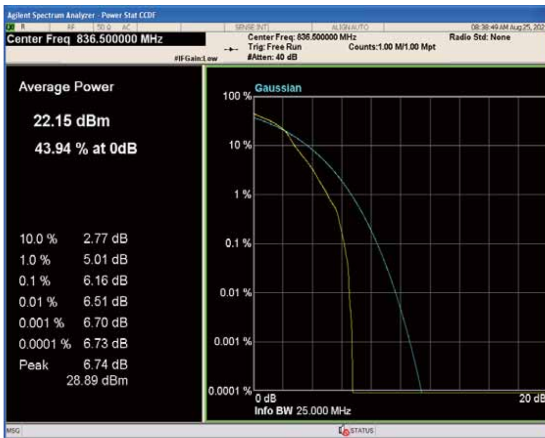
Band5 QPSK BW=10MHz Channel=20525 RB Size=1 Position=#0
