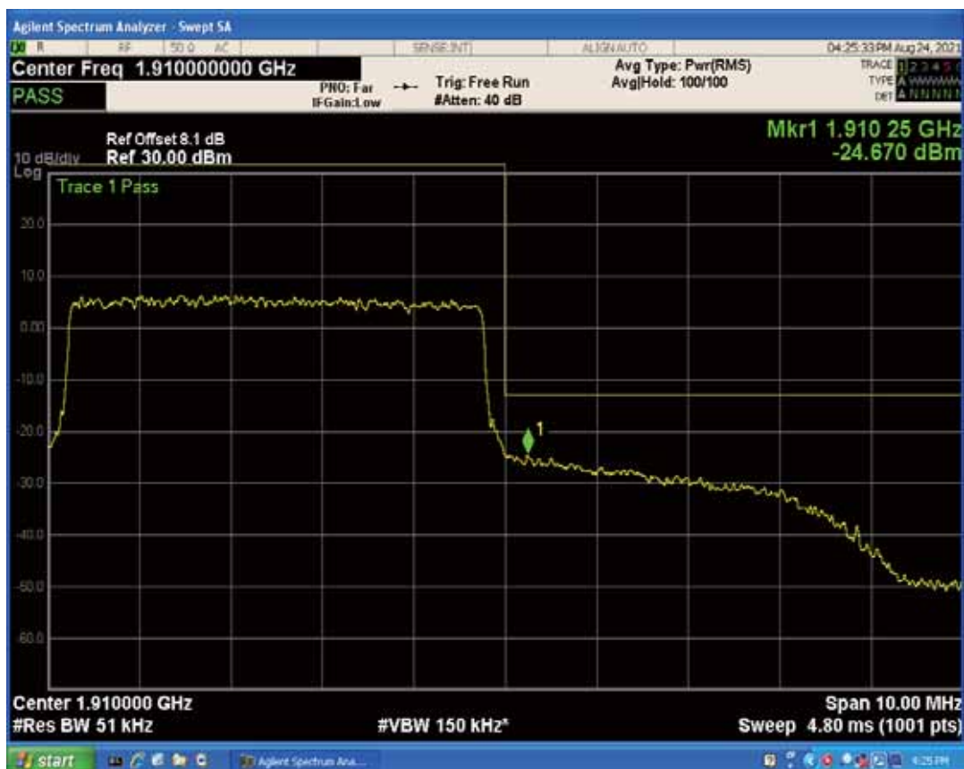
Band2 QAM16 BW=5MHz Channel=19175 RB Size=1 Position=#0
