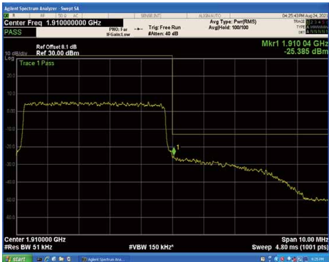
Band2 QAM16 BW=5MHz Channel=19175 RB Size=1 Position=#Max
