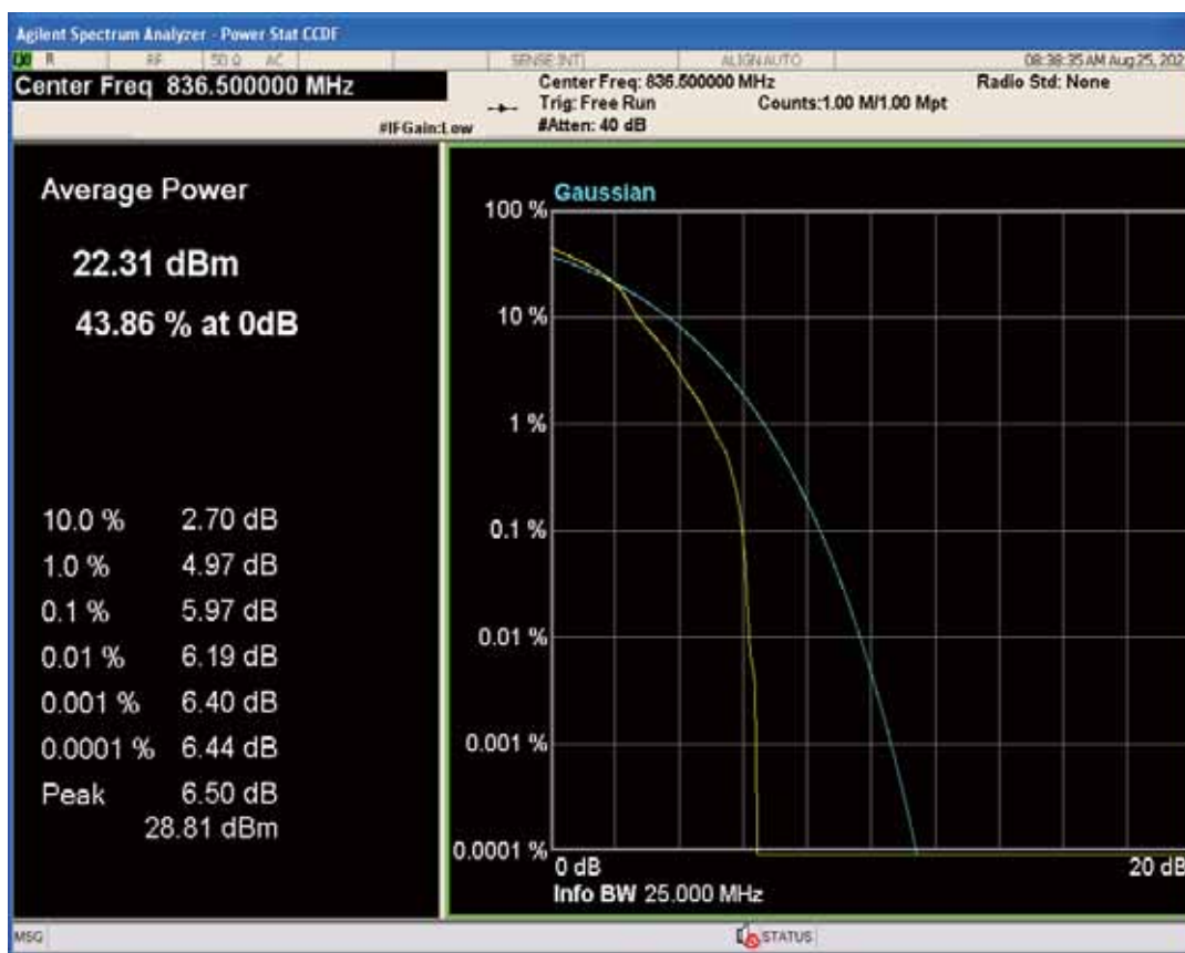
Band5 QAM16 BW=10MHz Channel=20525 RB Size=1 Position=#0
