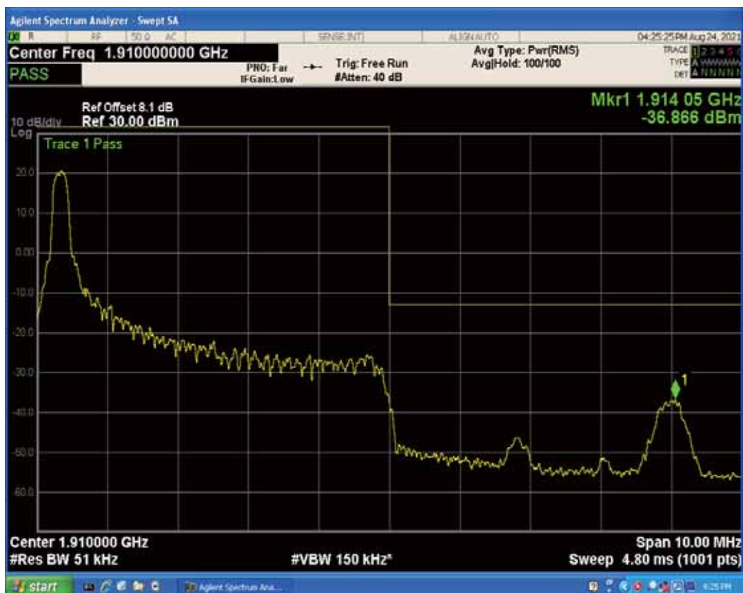
Band2 QPSK BW=5MHz Channel=19175 RB Size=1 Position=#Max
