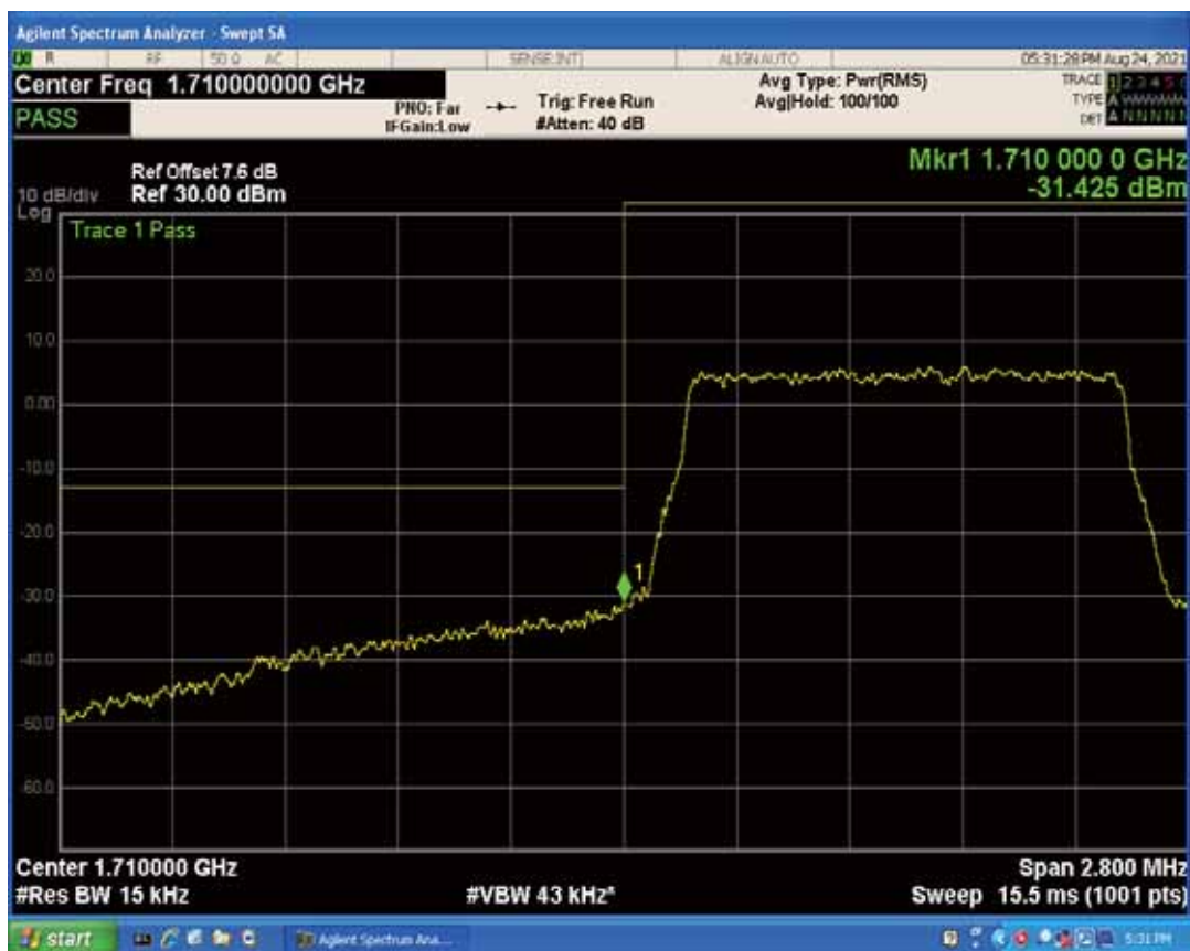
Band4 QPSK BW=1.4MHz Channel=20393 RB Size=1 Position=#Max
