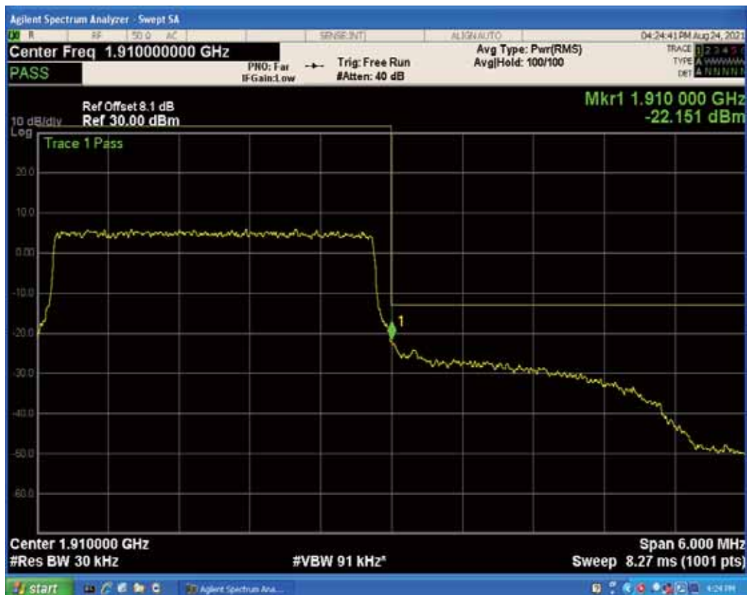
Band2 QAM16 BW=3MHz Channel=19185 RB Size=1 Position=#0
