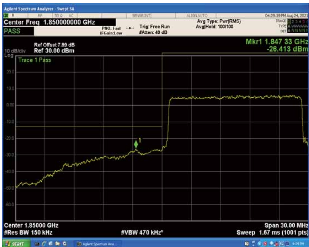
Band2 QPSK BW=15MHz Channel=18675 RB Size=1 Position=#Max
