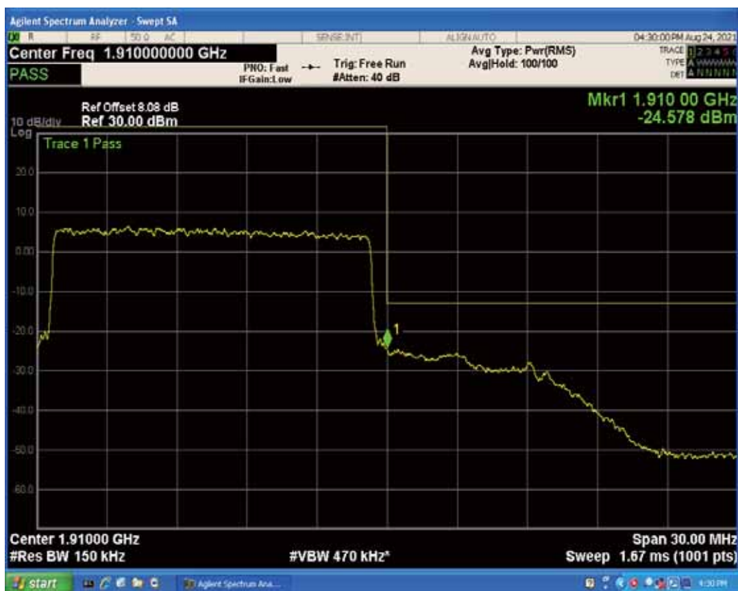
Band2 QPSK BW=15MHz Channel=19125 RB Size=1 Position=#Max
