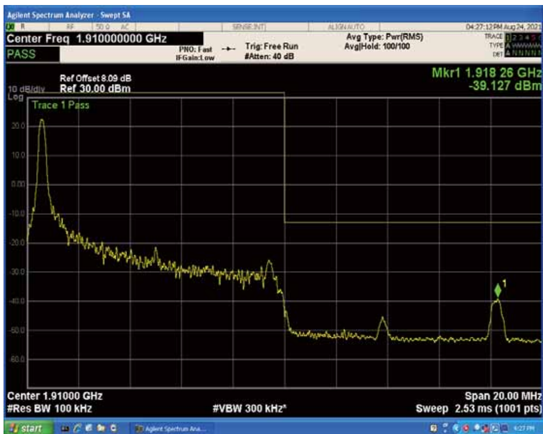
Band2 QPSK BW=10MHz Channel=19150 RB Size=1 Position=#Max
