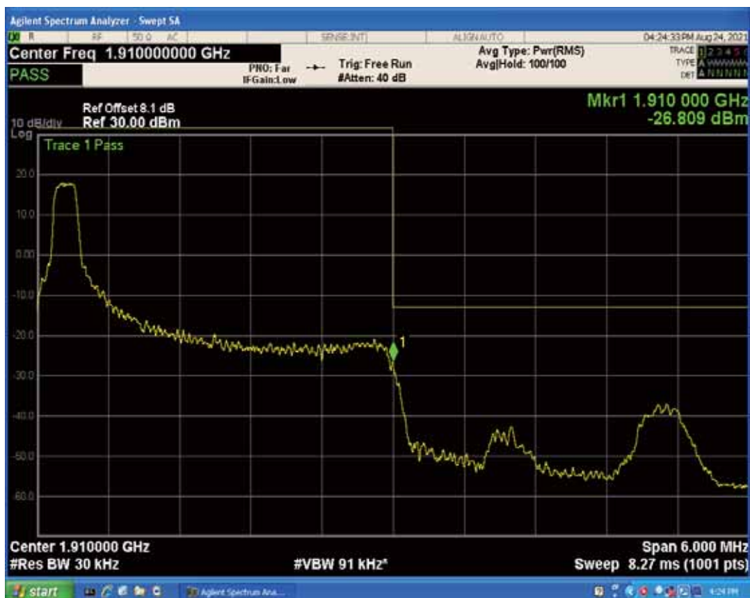
Band2 QPSK BW=3MHz Channel=19185 RB Size=1 Position=#Max
