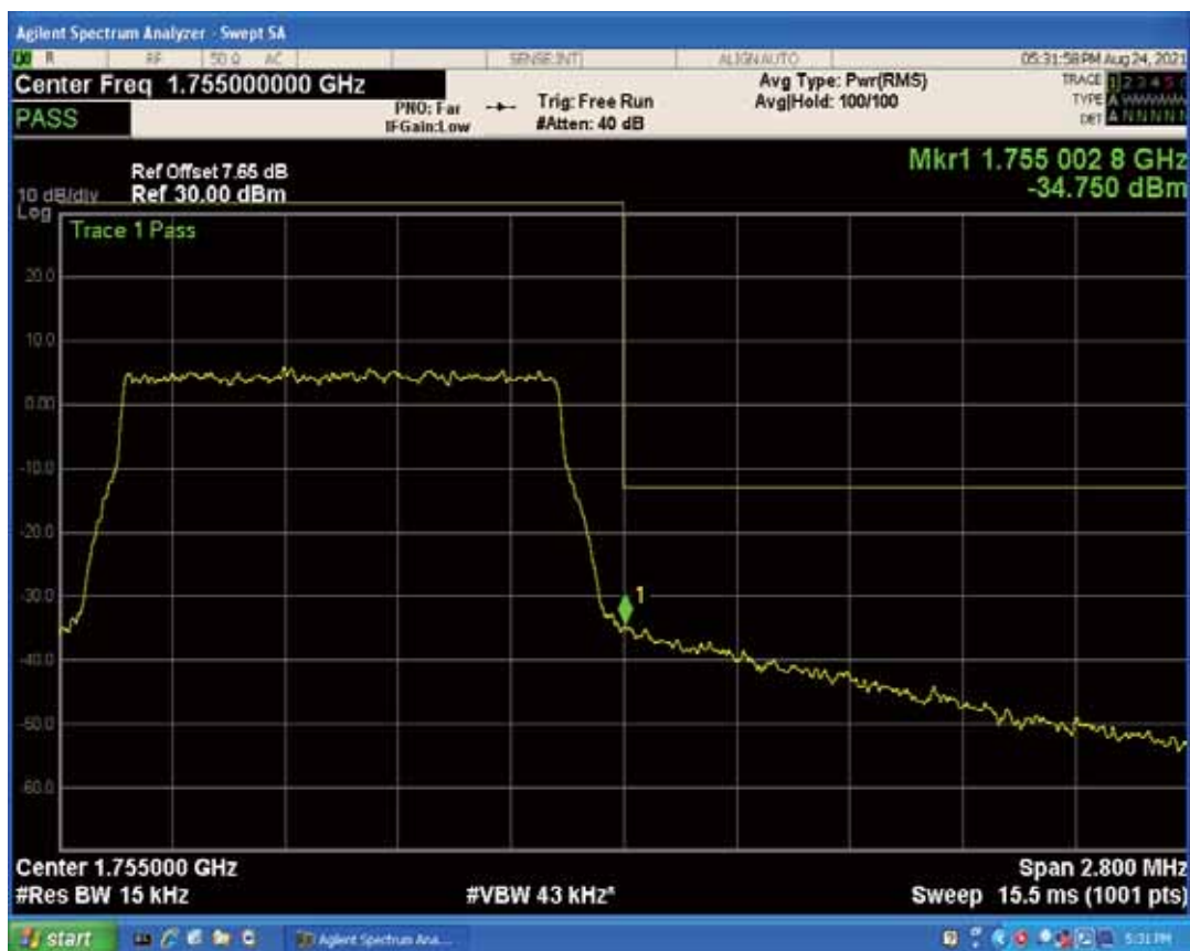
Band4 QPSK BW=3MHz Channel=19965 RB Size=1 Position=#Max
