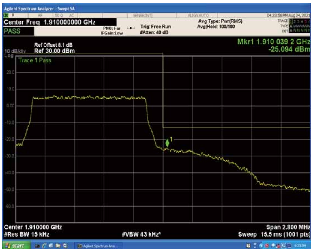
Band2 QAM16 BW=1.4MHz Channel=19193 RB Size=1 Position=#Max
