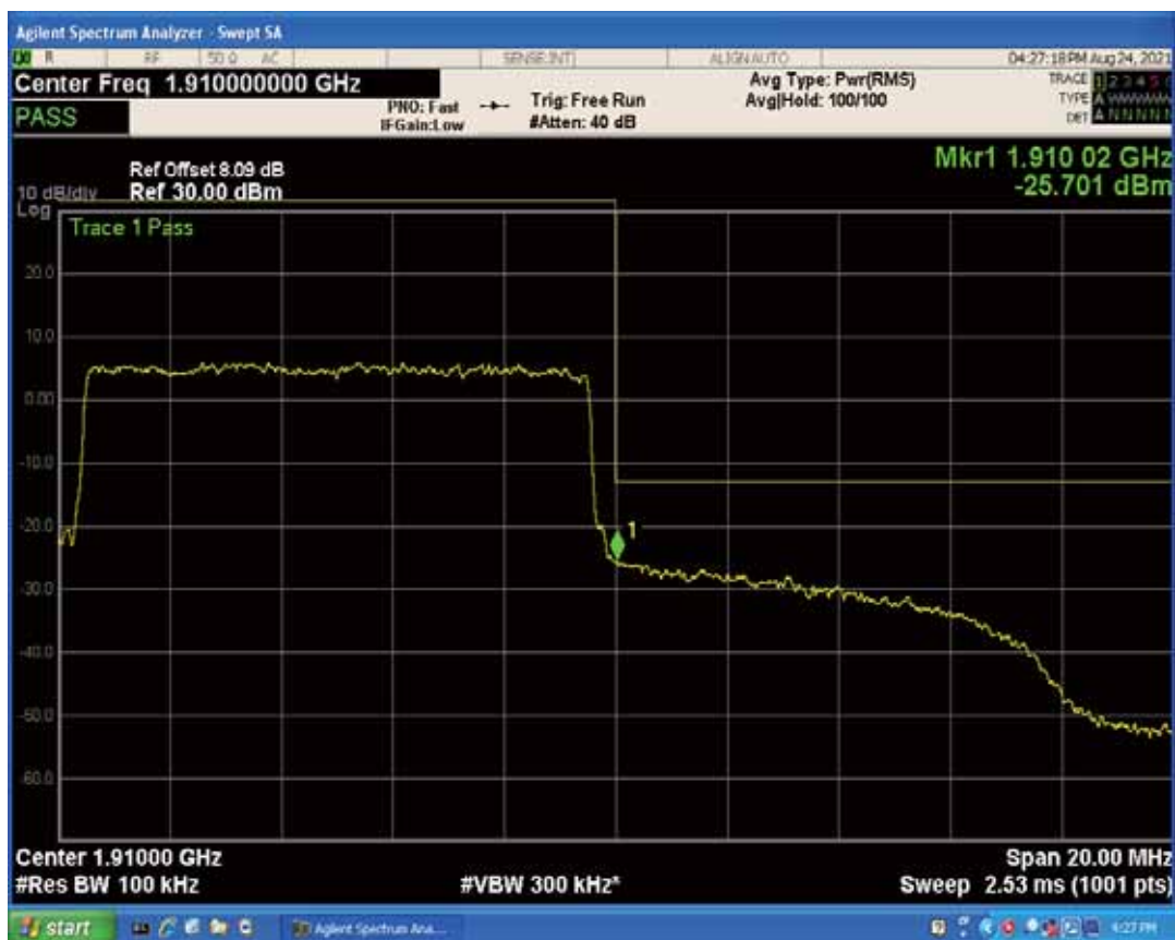
Band2 QAM16 BW=10MHz Channel=19150 RB Size=1 Position=#0
