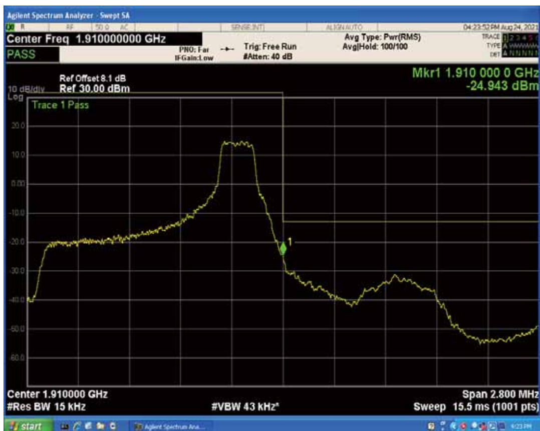
Band2 QPSK BW=3MHz Channel=18615 RB Size=1 Position=#0
