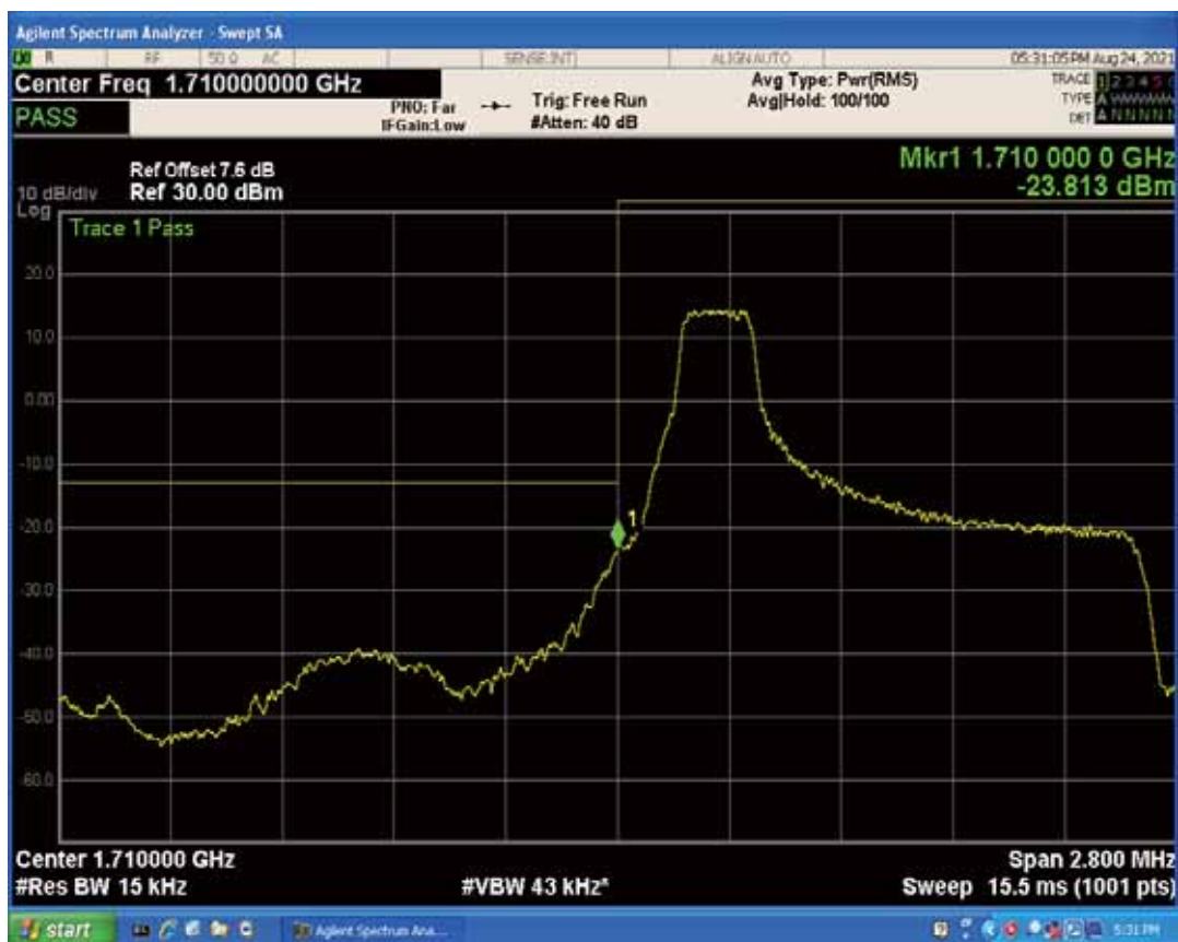
Band4 QPSK BW=1.4MHz Channel=19957 RB Size=1 Position=#Max
