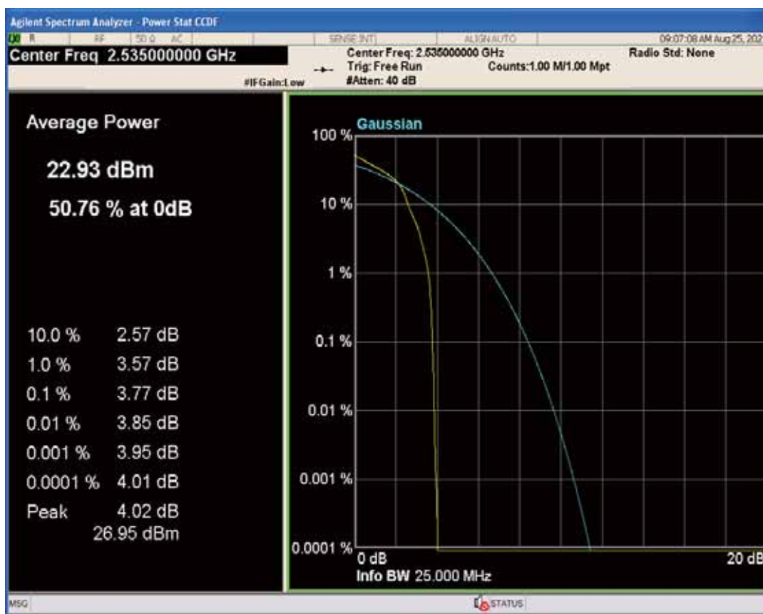
Band7 QPSK BW=15MHz Channel=21100 RB Size=1 Position=#0
