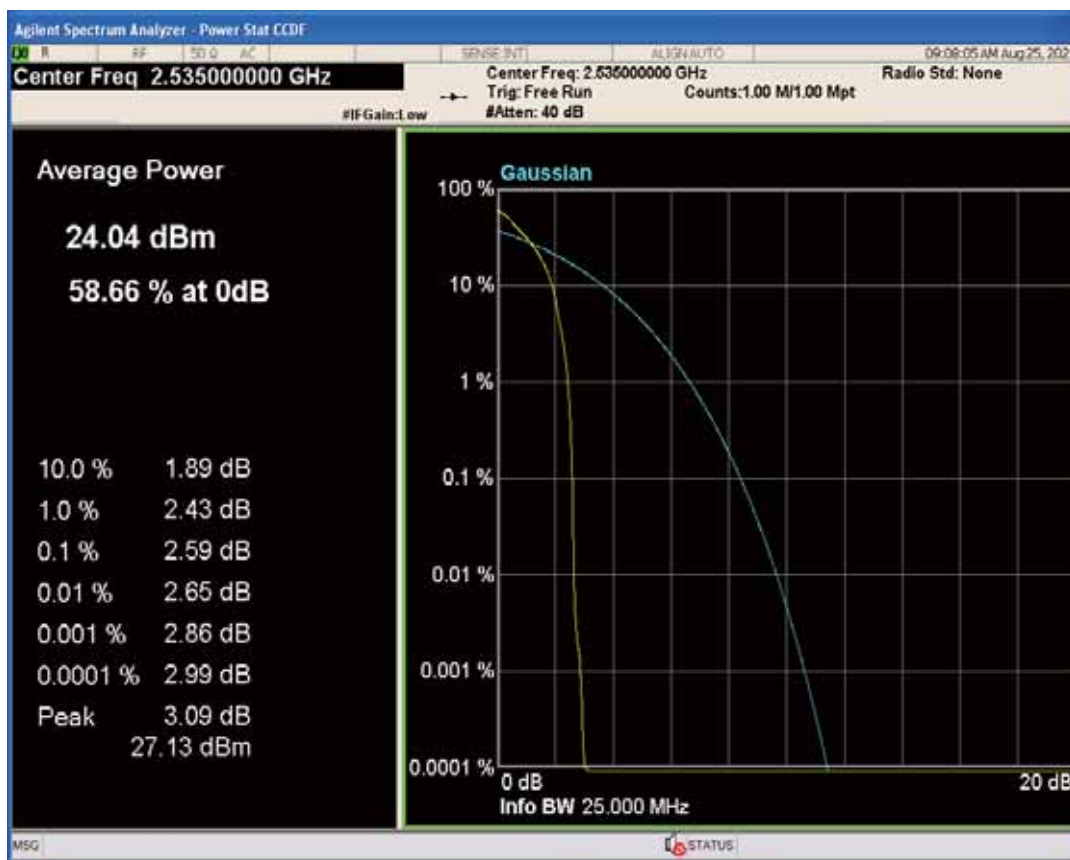
Band7 QAM16 BW=15MHz Channel=21100 RB Size=1 Position=#0
