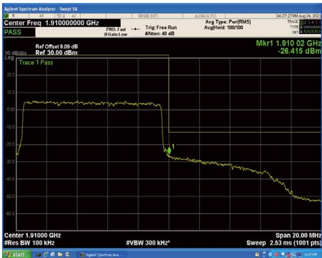
Band2 QAM16 BW=10MHz Channel=19150 RB Size=1 Position=#Max
