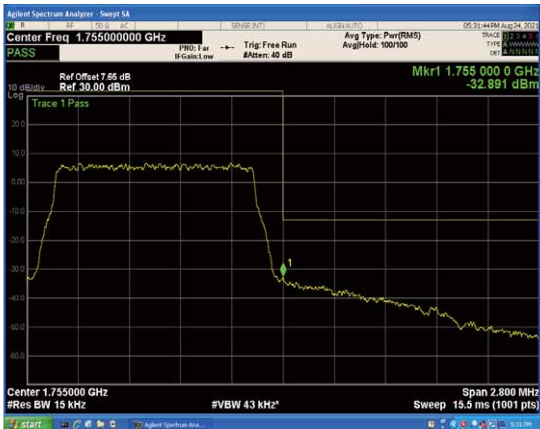
Band4 QAM16 BW=1.4MHz Channel=20393 RB Size=1 Position=#0
