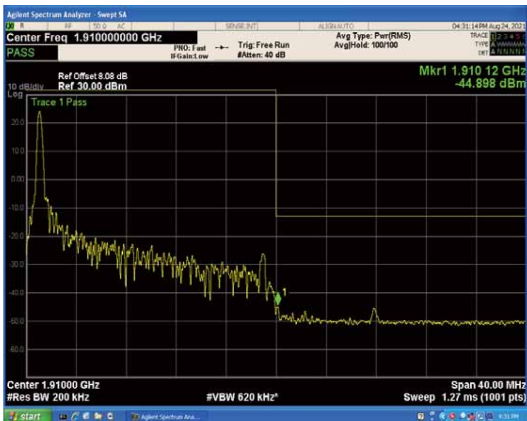
Band2 QPSK BW=20MHz Channel=19100 RB Size=1 Position=#Max
