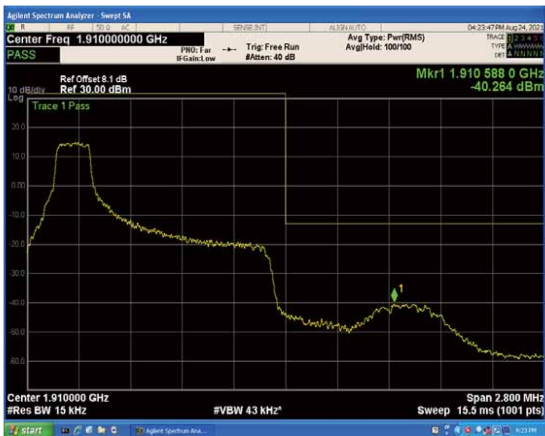
Band2 QAM16 BW=1.4MHz Channel=19193 RB Size=6 Position=#0
