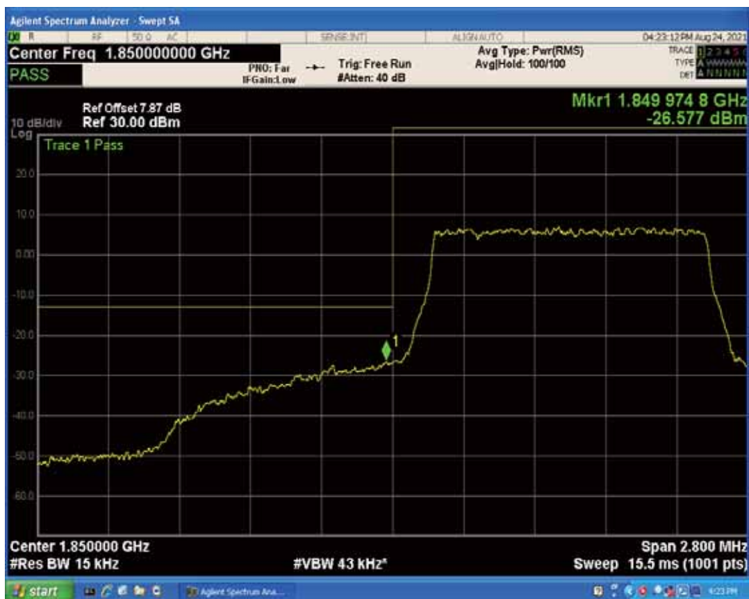
Band2 QAM16 BW=1.4MHz Channel=18607 RB Size=1 Position=#0
