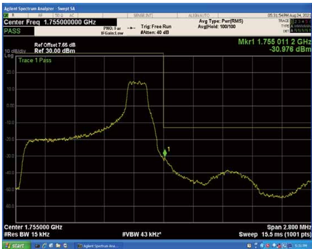
Band4 QPSK BW=3MHz Channel=19965 RB Size=1 Position=#0
