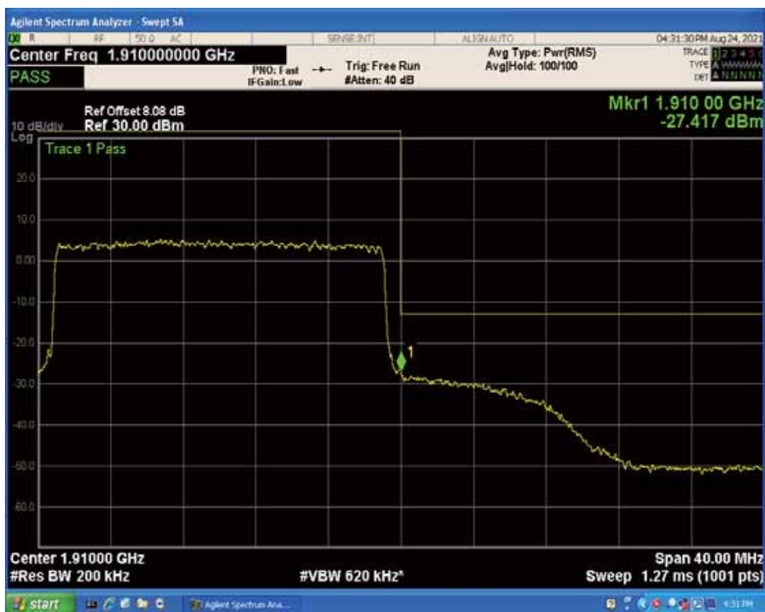
Band4 QPSK BW=1.4MHz Channel=19957 RB Size=1 Position=#0
