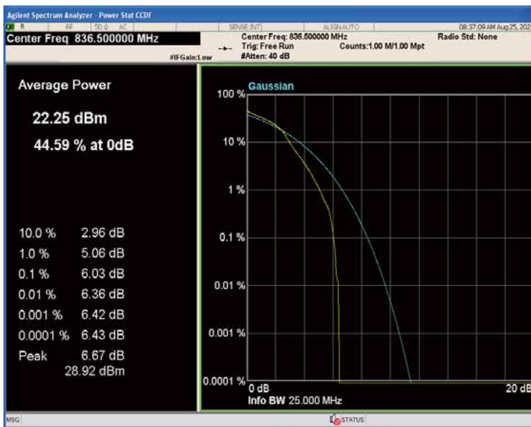
Band5 QAM16 BW=3MHz Channel=20525 RB Size=1 Position=#0
