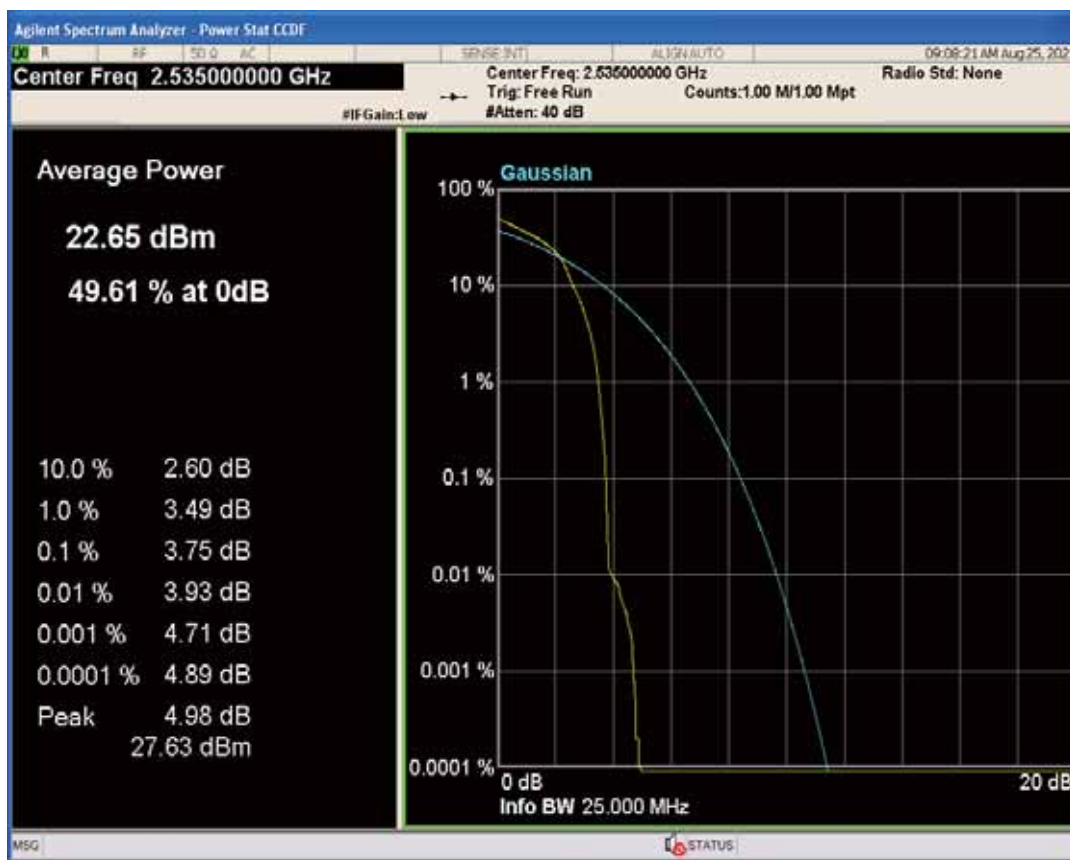
Band7 QPSK BW=20MHz Channel=21100 RB Size=1 Position=#0
