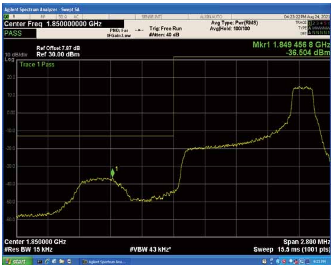
Band2 QPSK BW=1.4MHz Channel=19193 RB Size=1 Position=#0
