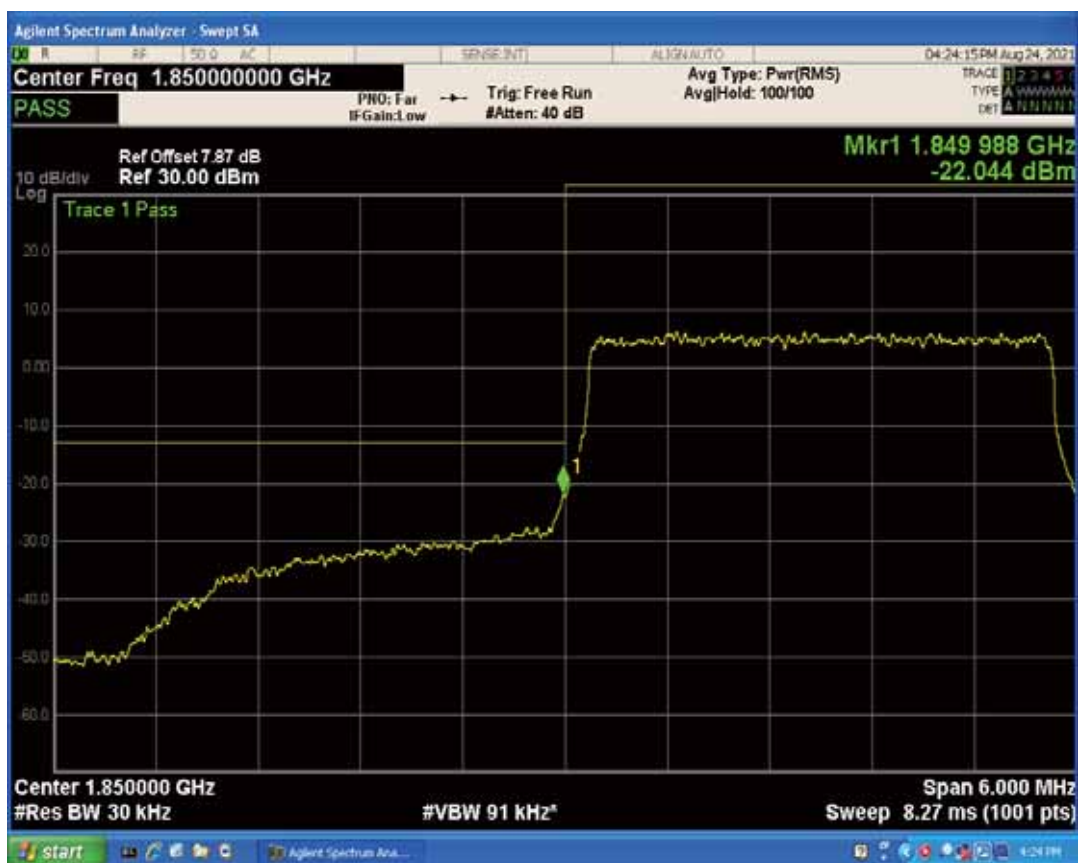
Band2 QPSK BW=3MHz Channel=18615 RB Size=1 Position=#Max
