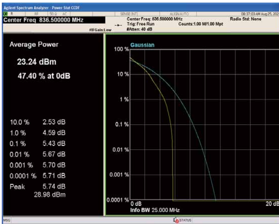
Band5 QAM16 BW=1.4MHz Channel=20525 RB Size=1 Position=#0
