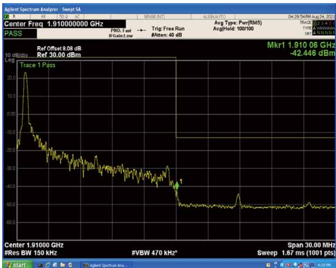
Band2 QPSK BW=15MHz Channel=19125 RB Size=75 Position=#0
