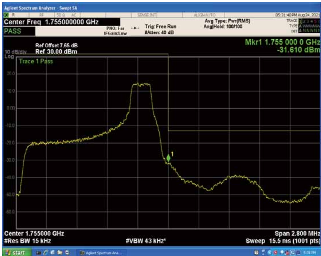
Band4 QPSK BW=1.4MHz Channel=20393 RB Size=6 Position=#0
