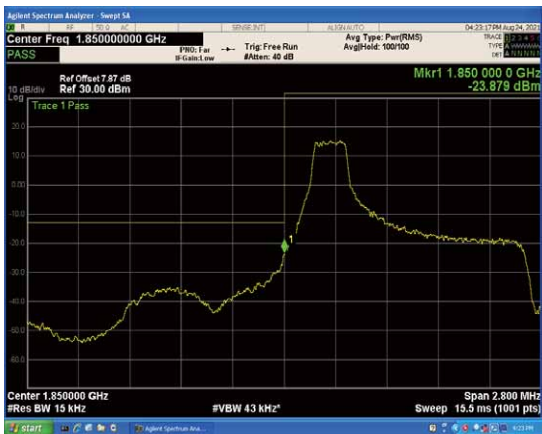
Band2 QAM16 BW=1.4MHz Channel=18607 RB Size=6 Position=#0
