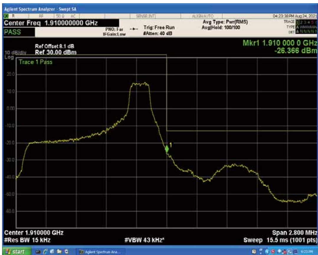
Band2 QPSK BW=1.4MHz Channel=19193 RB Size=6 Position=#0
