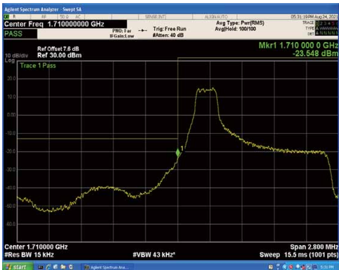
Band4 QPSK BW=1.4MHz Channel=19957 RB Size=6 Position=#0
