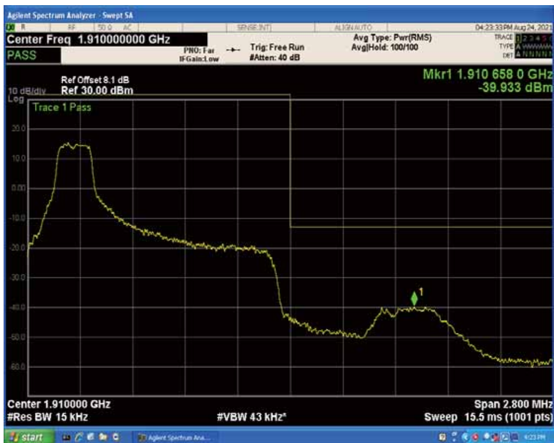
Band2 QPSK BW=1.4MHz Channel=19193 RB Size=1 Position=#Max
