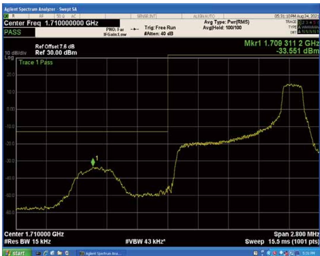
Band4 QAM16 BW=1.4MHz Channel=19957 RB Size=1 Position=#0
