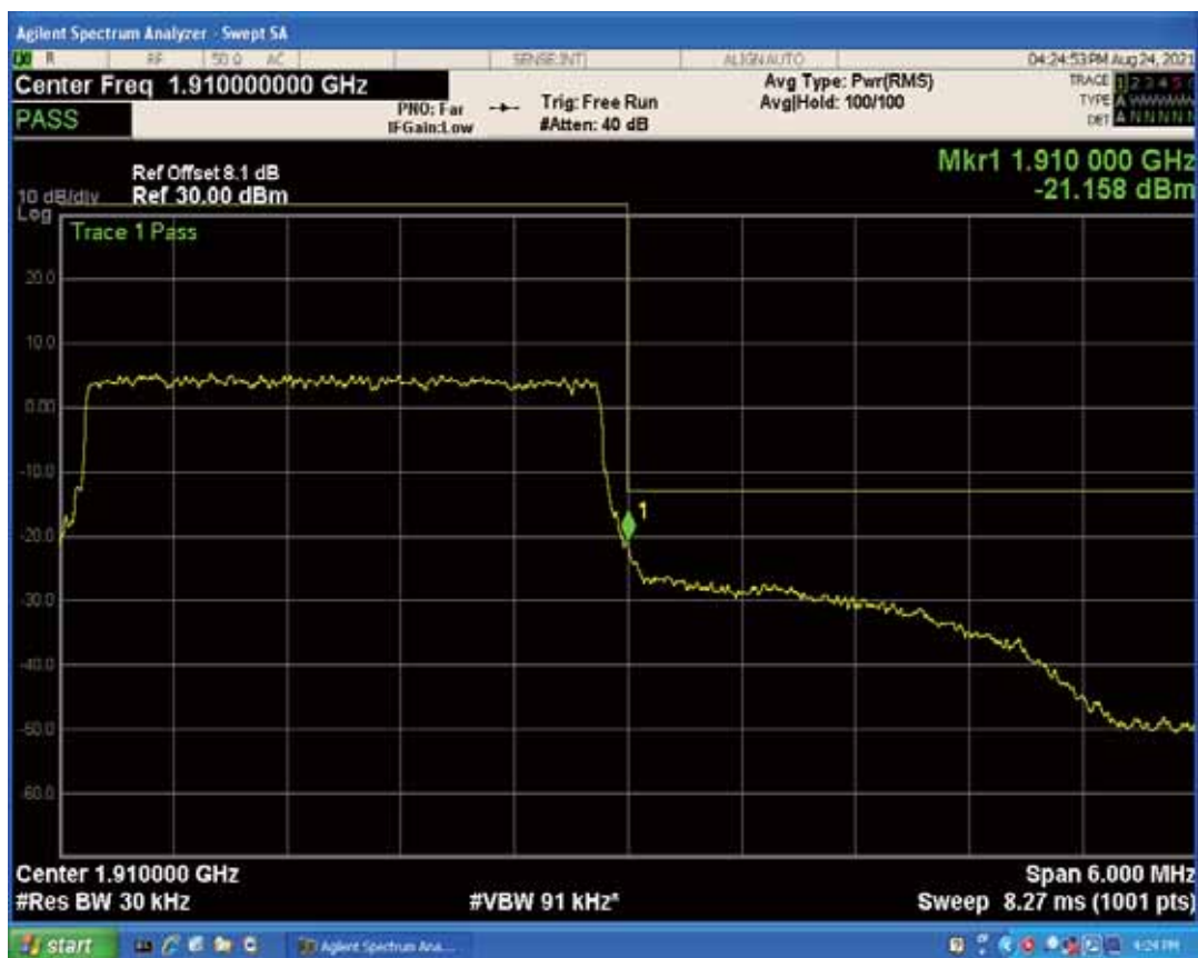
Band2 QAM16 BW=3MHz Channel=19185 RB Size=1 Position=#Max
