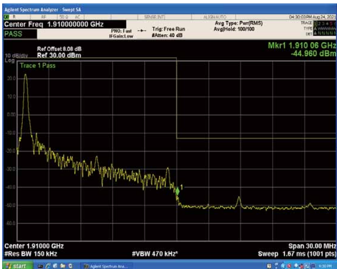
Band2 QAM16 BW=15MHz Channel=19125 RB Size=1 Position=#Max
