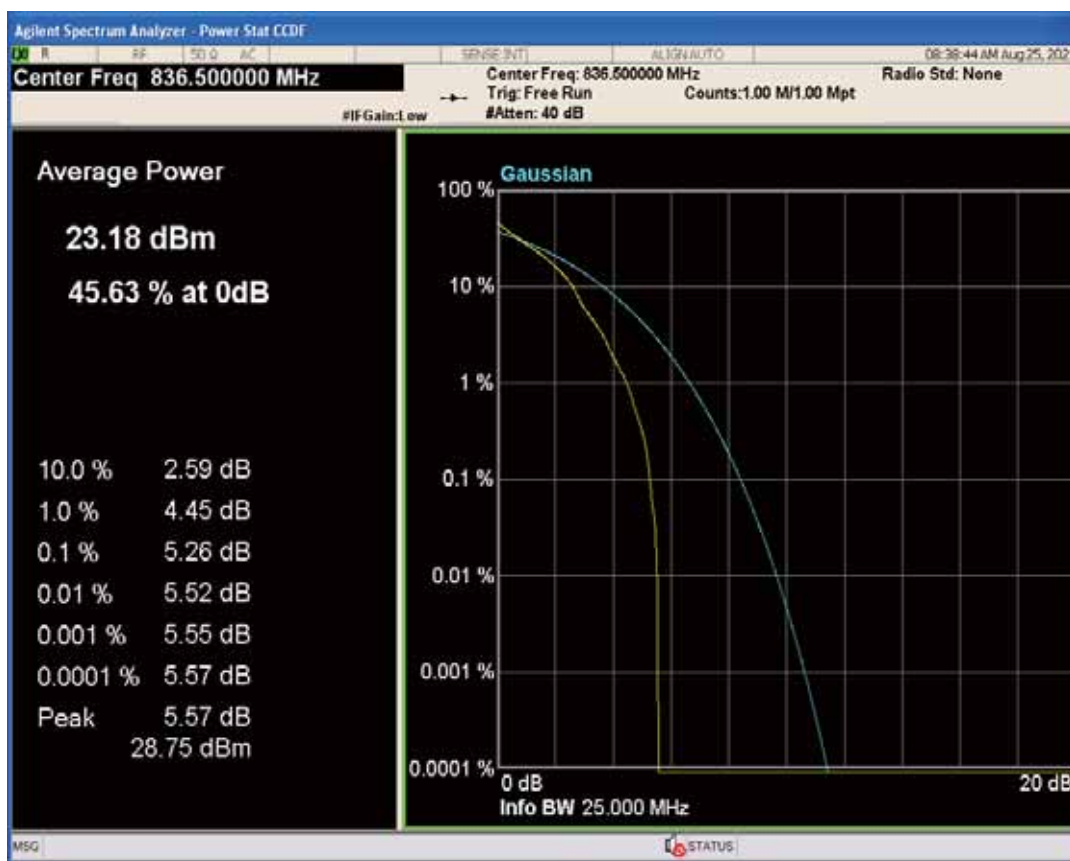
Band7 QPSK BW=5MHz Channel=21100 RB Size=1 Position=#0
