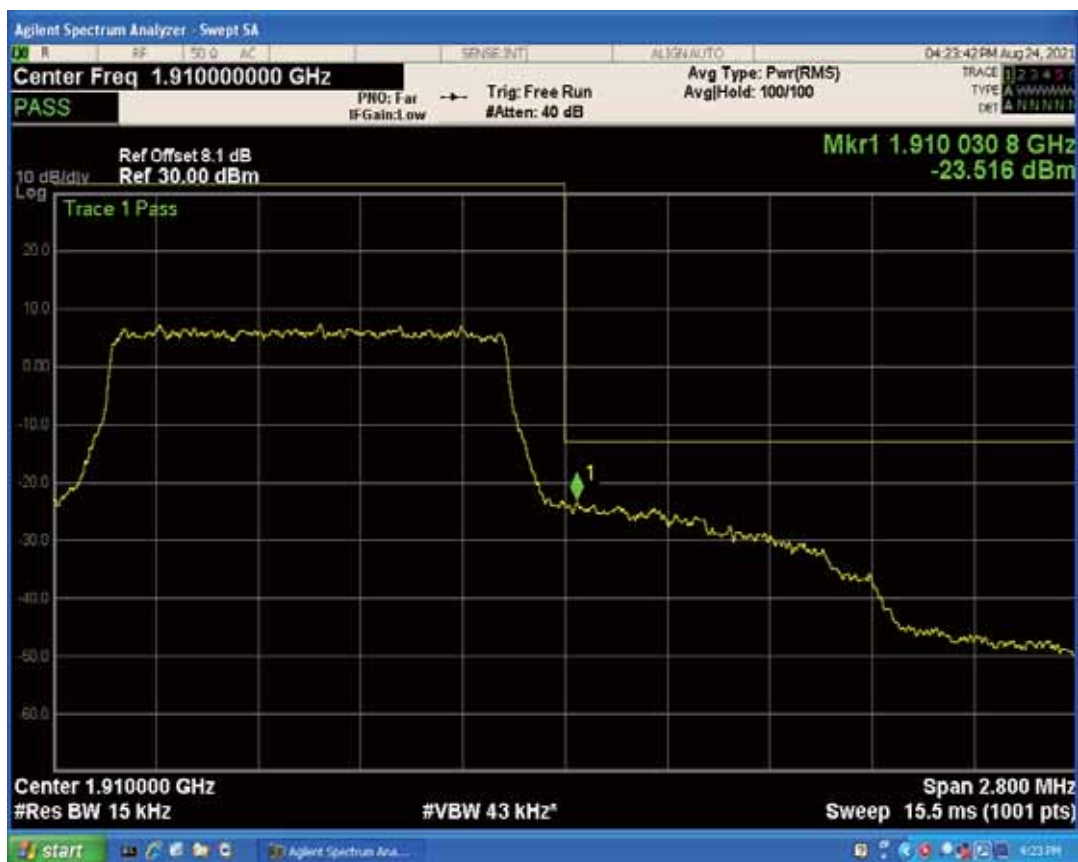
Band2 QAM16 BW=1.4MHz Channel=19193 RB Size=1 Position=#0
