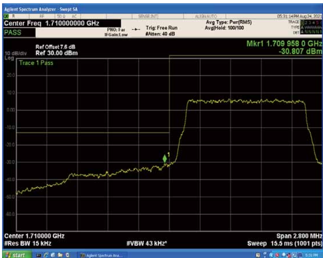
Band4 QAM16 BW=1.4MHz Channel=19957 RB Size=1 Position=#Max
