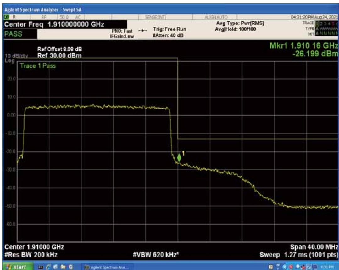
Band2 QAM16 BW=20MHz Channel=19100 RB Size=1 Position=#Max
