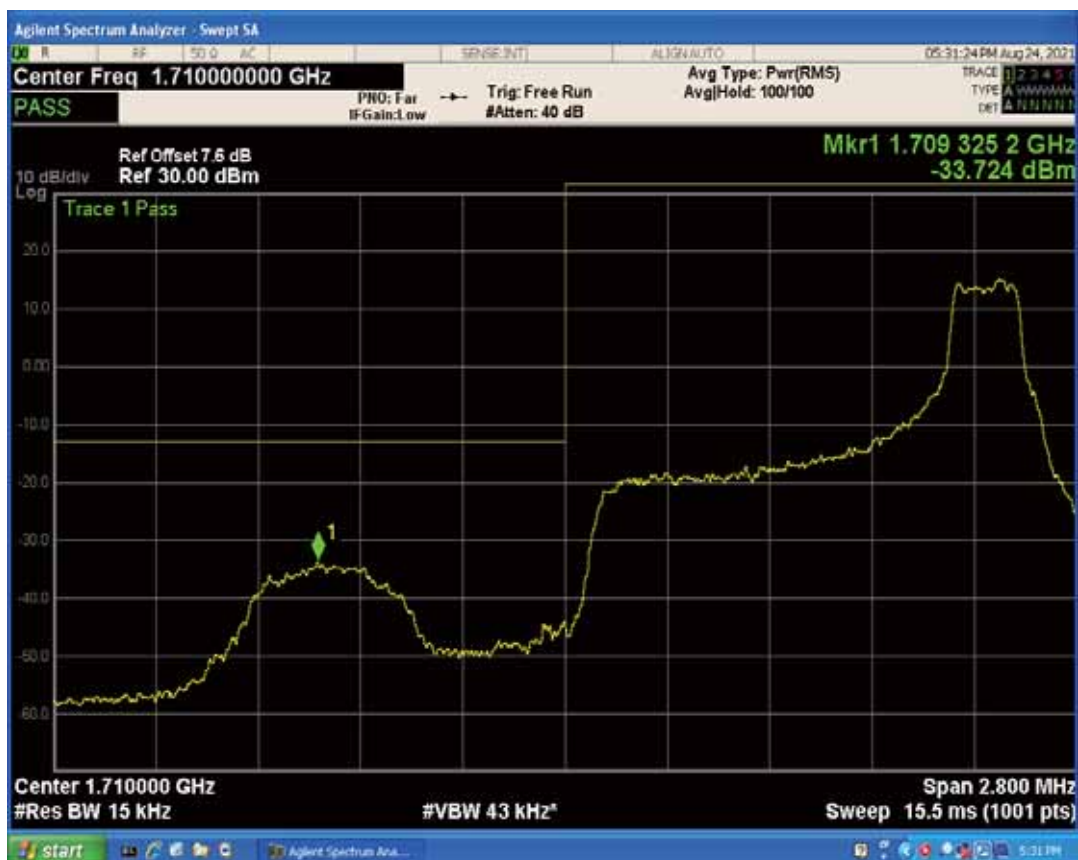
Band4 QPSK BW=1.4MHz Channel=20393 RB Size=1 Position=#0
