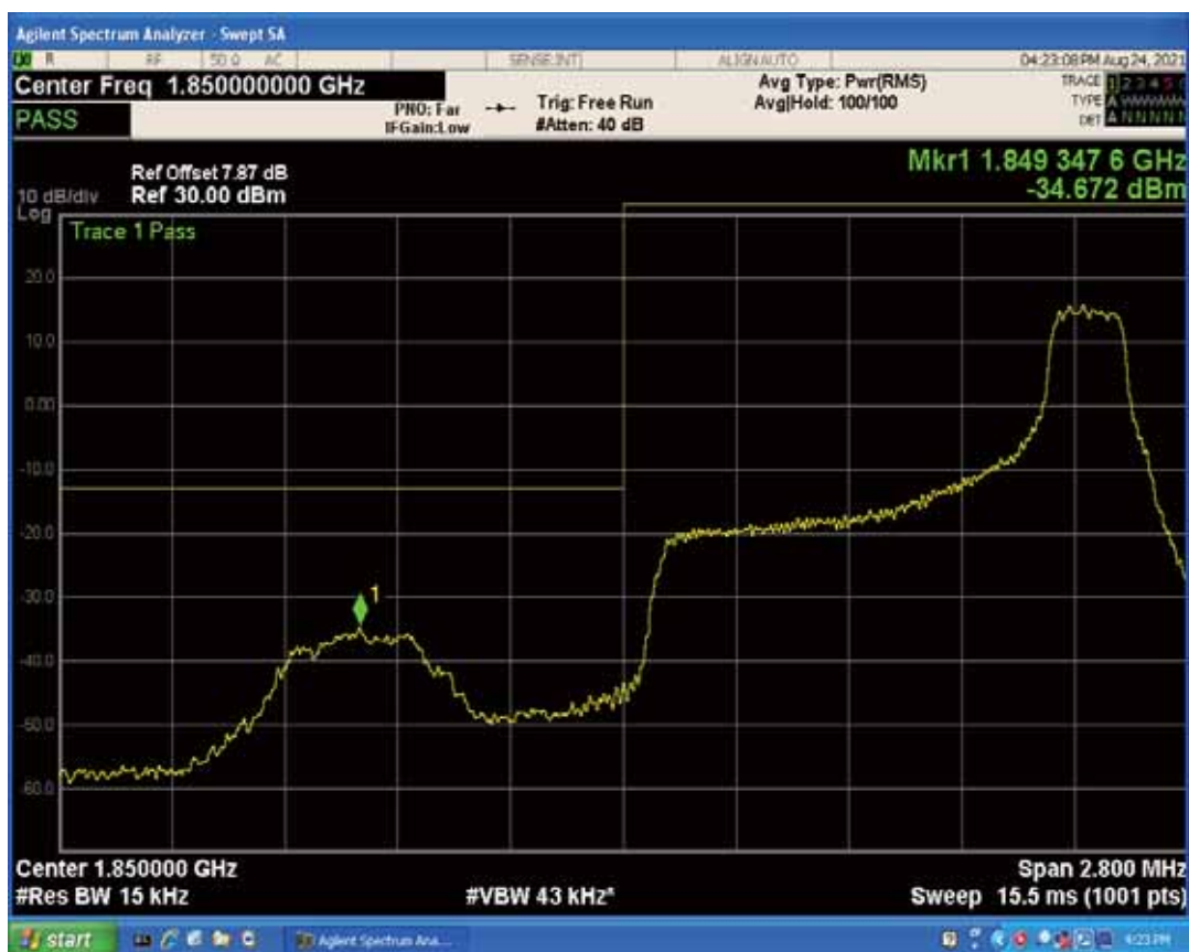
Band2 QPSK BW=1.4MHz Channel=18607 RB Size=6 Position=#0
