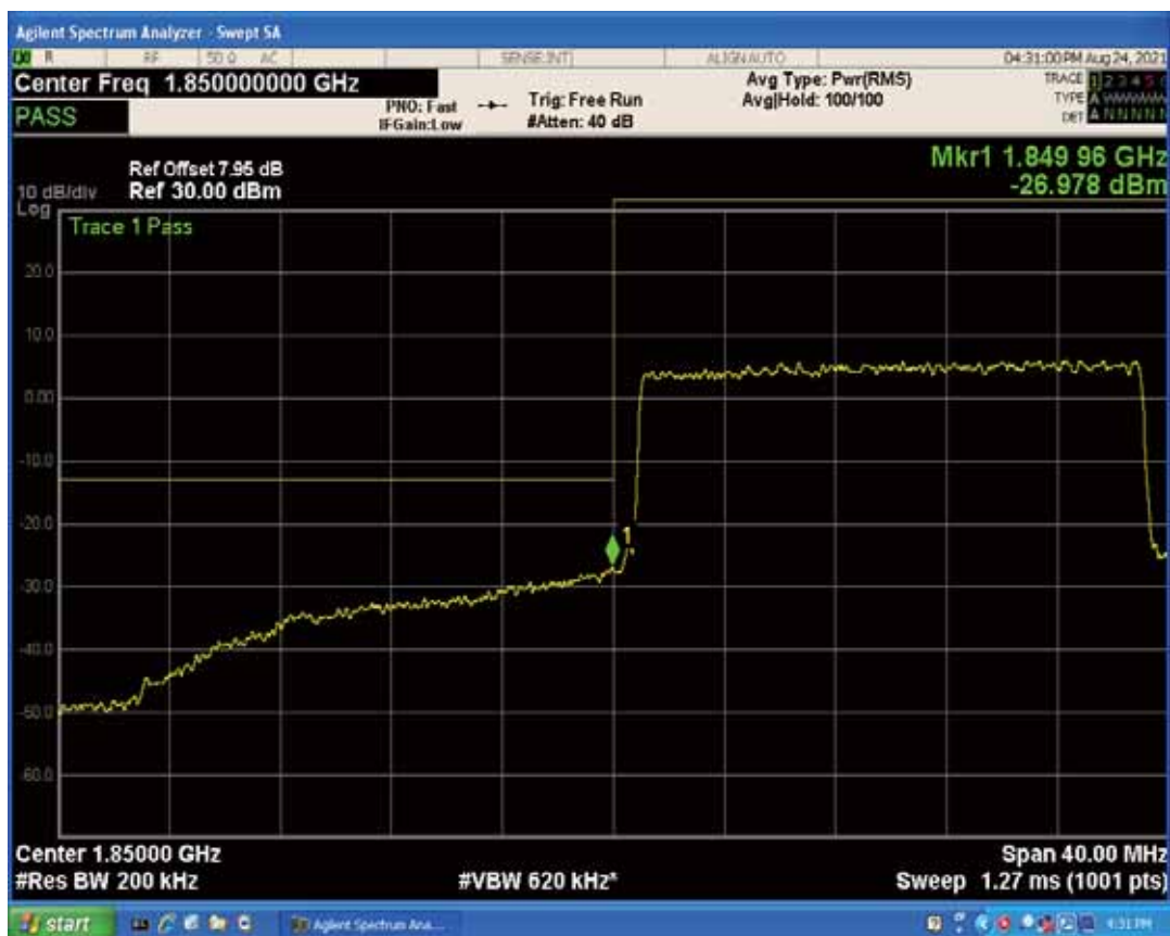
Band2 QAM16 BW=20MHz Channel=18700 RB Size=1 Position=#0
