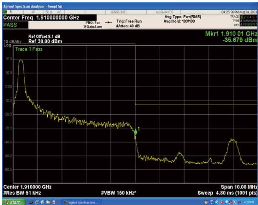
Band2 QAM16 BW=5MHz Channel=19175 RB Size=25 Position=#0
