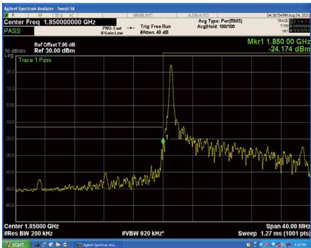
Band2 QPSK BW=20MHz Channel=18700 RB Size=1 Position=#Max
