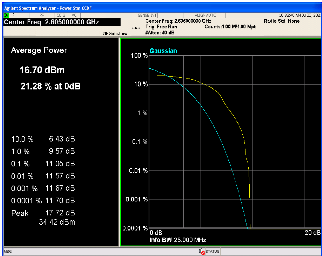
Band41 QAM16 BW=20MHz Channel=40740 RB Size=1 Position=#0
