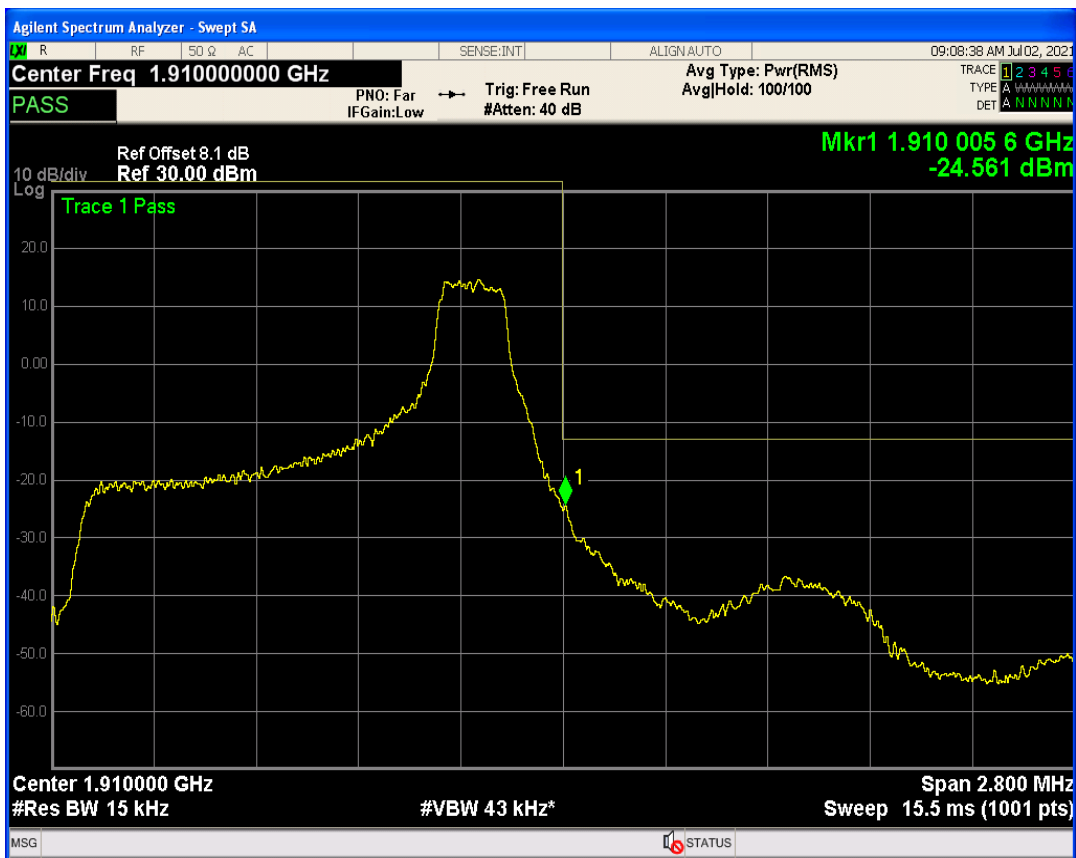
Band2 QPSK BW=3MHz Channel=18615 RB Size=1 Position=#Max
