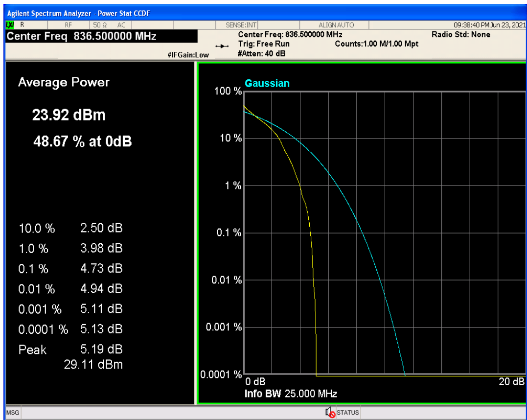
Band5 QAM16 BW=10MHz Channel=20525 RB Size=1 Position=#0
