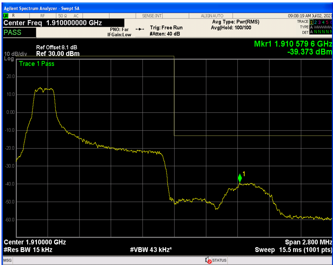
Band2 QPSK BW=1.4MHz Channel=19193 RB Size=1 Position=#Max
