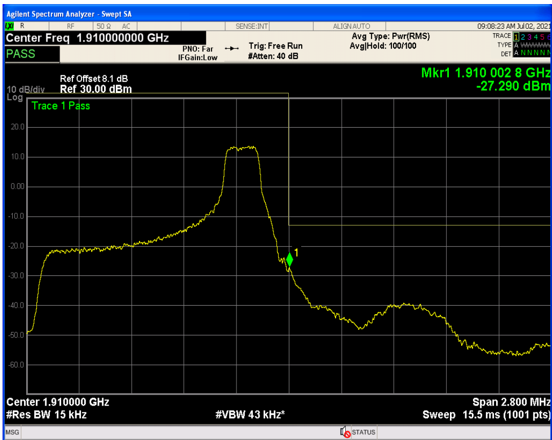
Band2 QPSK BW=1.4MHz Channel=19193 RB Size=6 Position=#0
