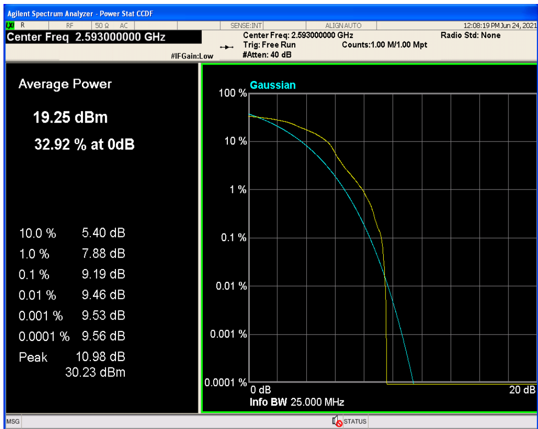
Band41 QPSK BW=15MHz Channel=40620 RB Size=1 Position=#0
