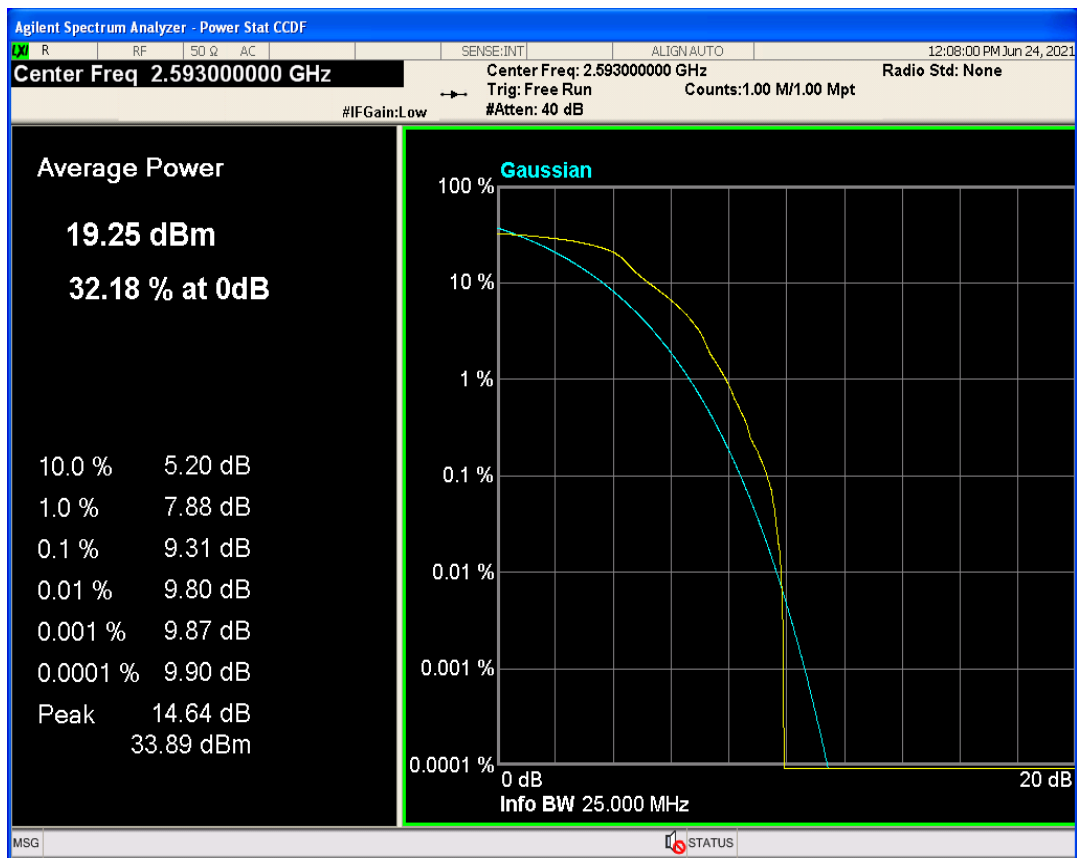
Band41 QAM16 BW=10MHz Channel=40620 RB Size=1 Position=#0
