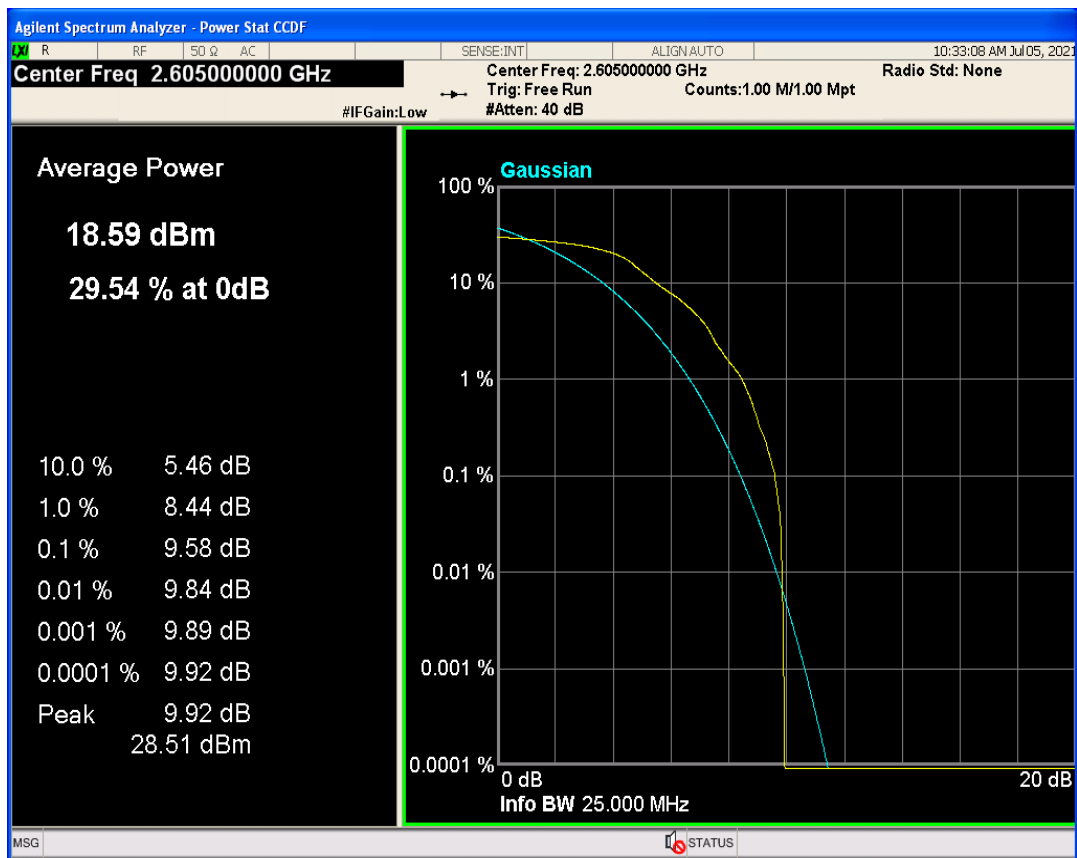
Band41 QAM16 BW=5MHz Channel=40740 RB Size=1 Position=#0
