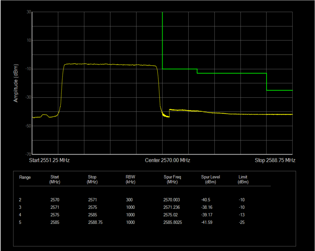
LTE Band7 QAM16 BW=15MHz Channel=21375 RB Size=1 Position=#0
