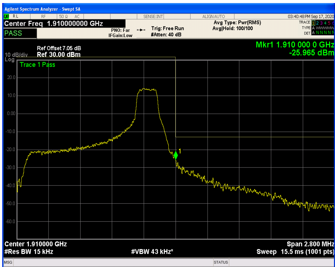
LTE Band2 QAM16 BW=1.4MHz Channel=19193 RB Size=1 Position=#0
