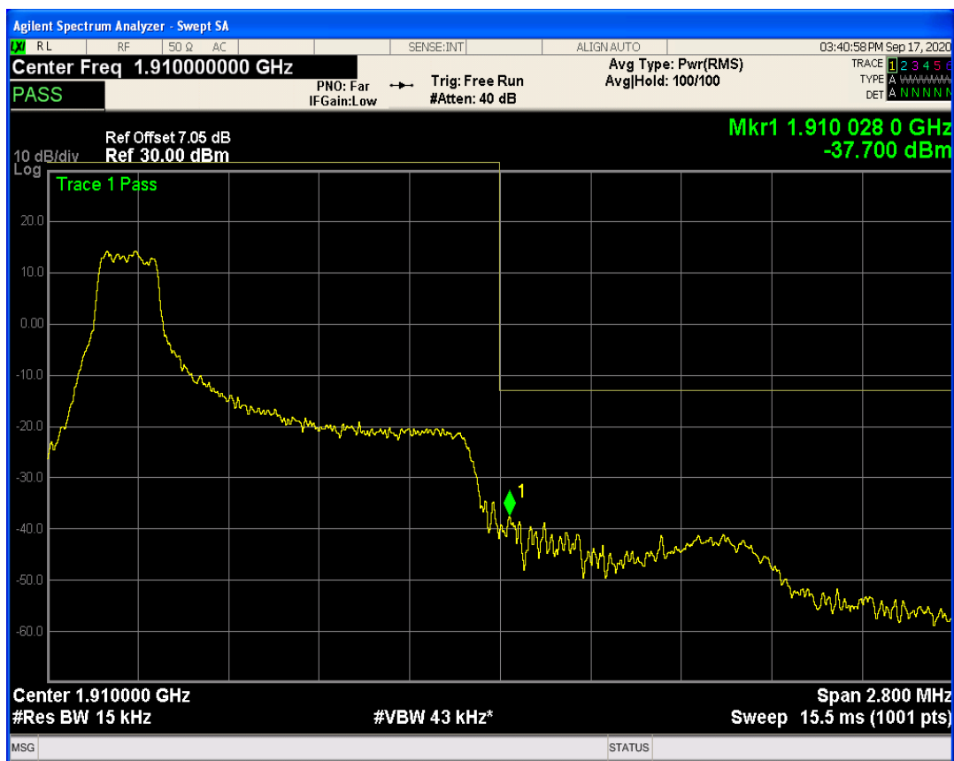
LTE Band2 QPSK BW=1.4MHz Channel=19193 RB Size=6 Position=#0
