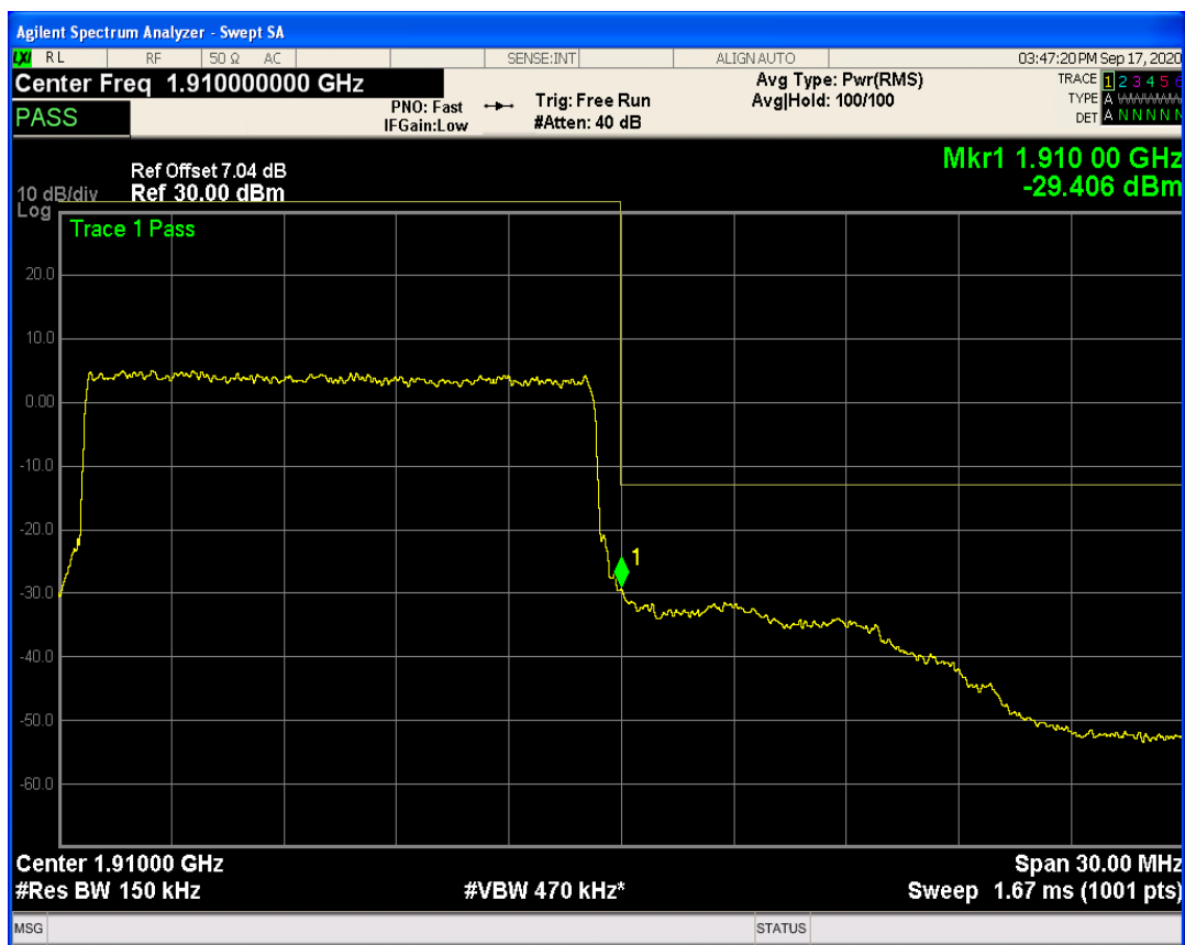
LTE Band2 QAM16 BW=15MHz Channel=19125 RB Size=1 Position=#0
