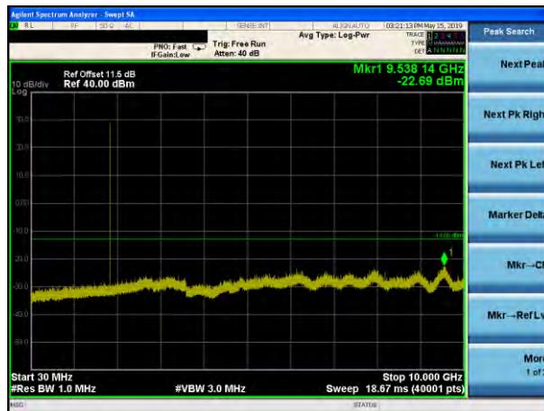
Conducted Emission Transmitting Mode CH 251
