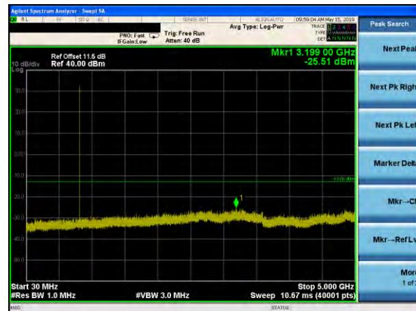
Conducted Emission Transmitting Mode CH 128
