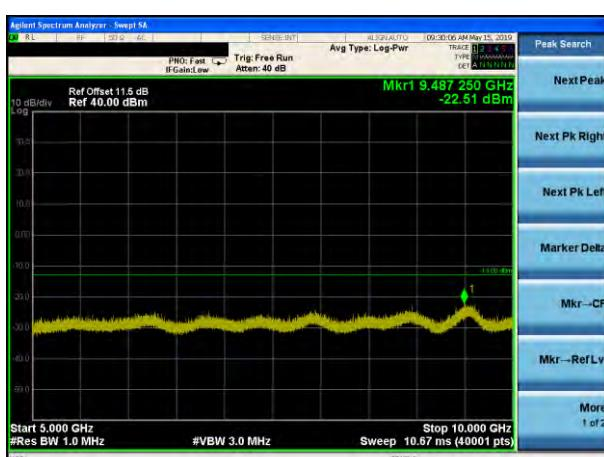
Conducted Emission Transmitting Mode CH 512
