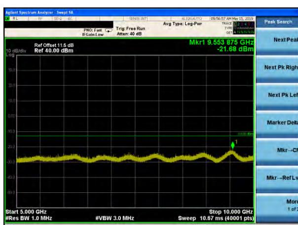
Conducted Emission Transmitting Mode CH 190
