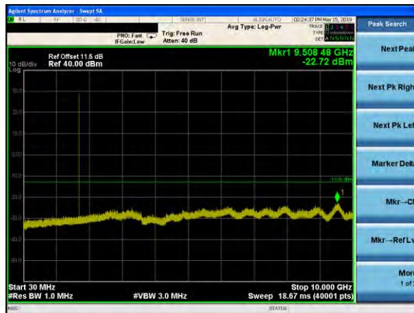
Conducted Emission Transmitting Mode CH 251
