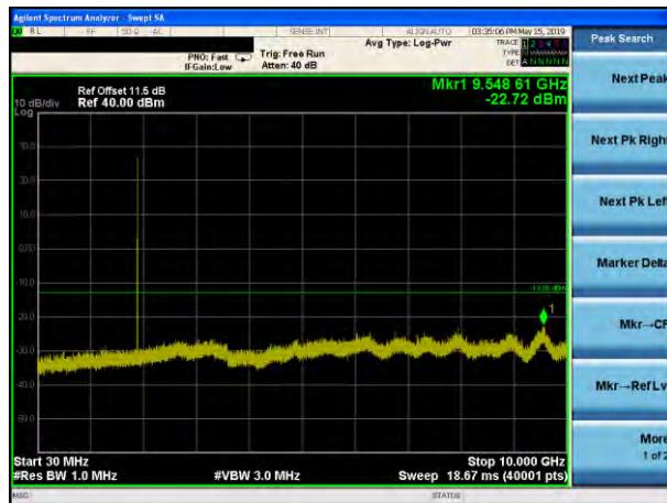
Conducted Emission Transmitting Mode CH 661
