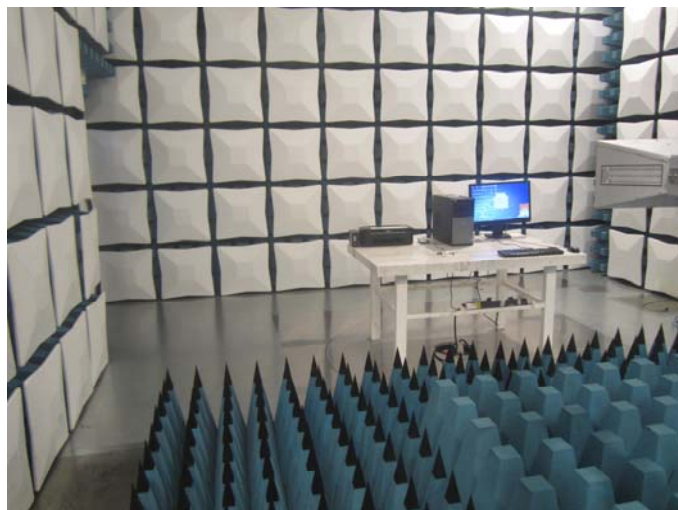
Radiated Emission (above 1GHz) Connect to PC
