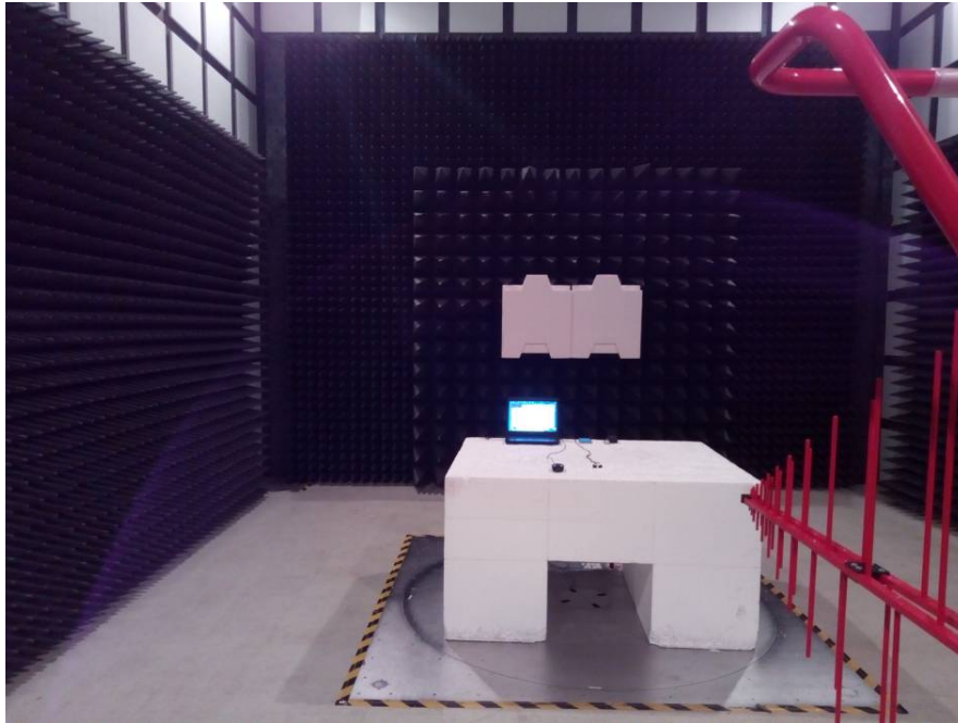
Radiated Emissions – Front View (Below 1 GHz)
