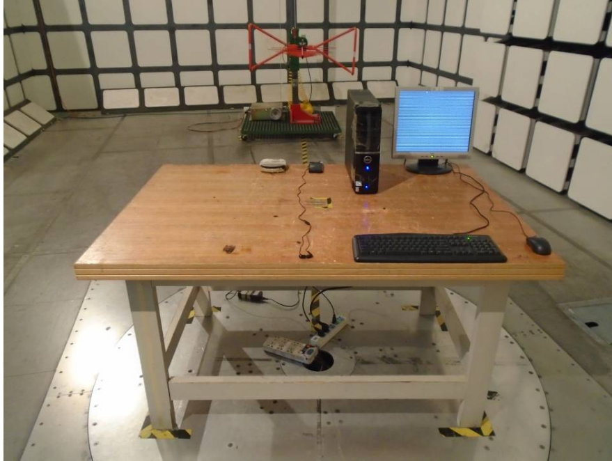
Radiated Emissions – Front View (Below 1 GHz)
