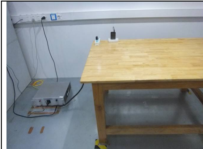
Conducted Emissions Test Setup Front View
