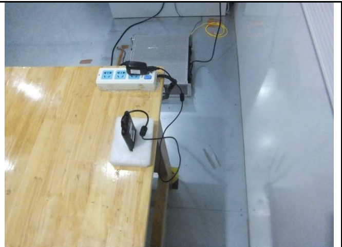
Conducted Emissions Test Setup Side View
