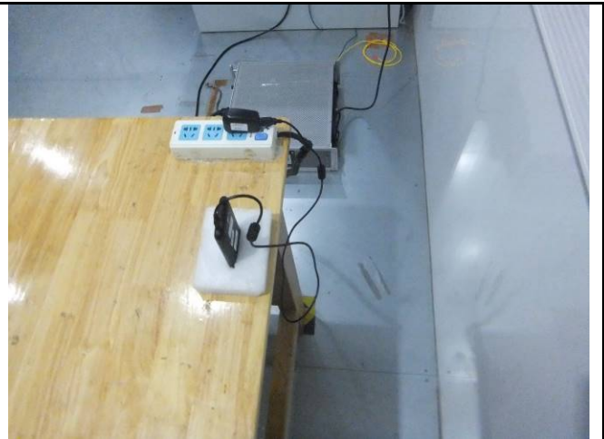
Conducted Emissions Test Setup Side View
