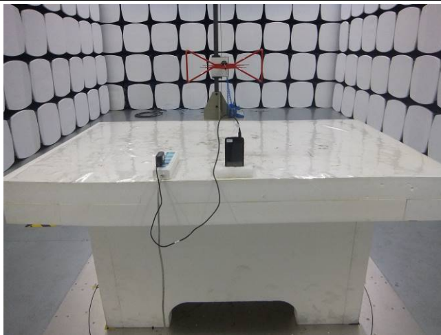
Conducted Emissions Test Setup Front View
