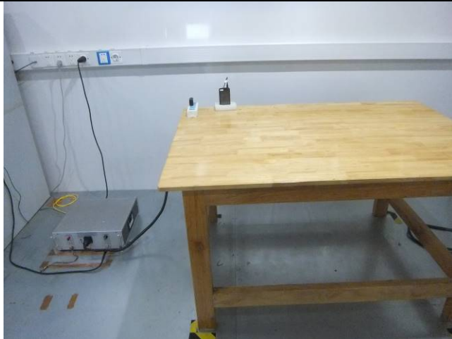
Conducted Emissions Test Setup Front View
