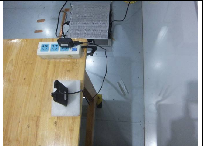
Conducted Emissions Test Setup Side View
