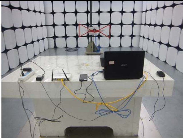
Radiated Spurious Emissions Test Setup Below 1GHz
