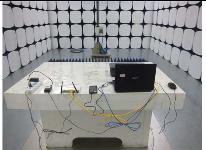
Radiated Spurious Emissions Test Setup Above 1GHz
