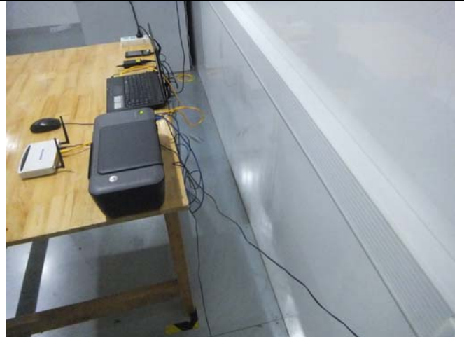
Conducted Emissions Test Setup – Side View
