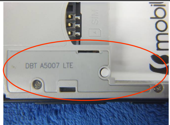
LTE- Antenna View
