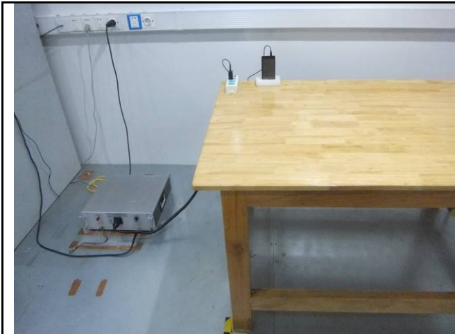
Conducted Emissions Test Setup Front View
