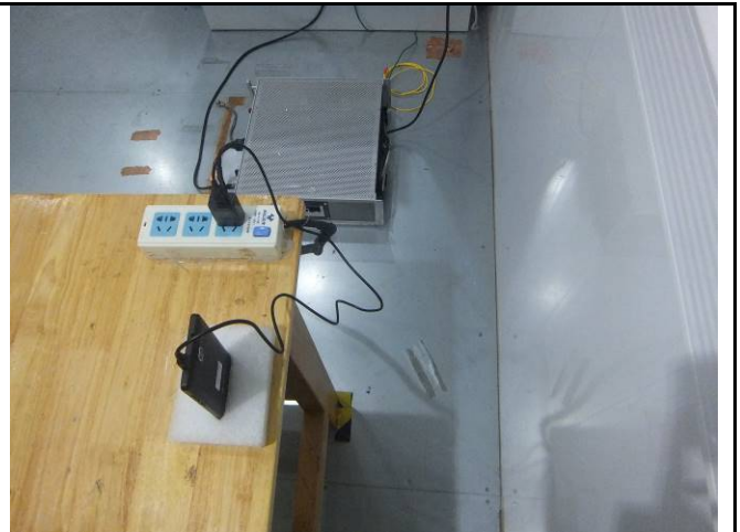
Conducted Emissions Test Setup Side View
