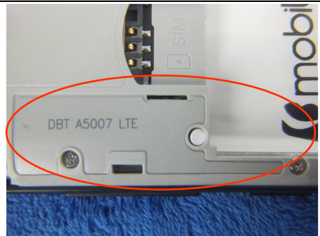
LTE- Antenna View
