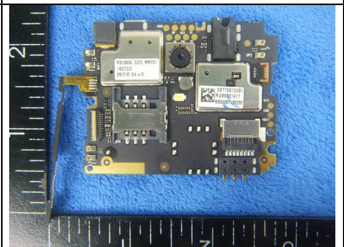
Mainboard with Shielding - Rear View
