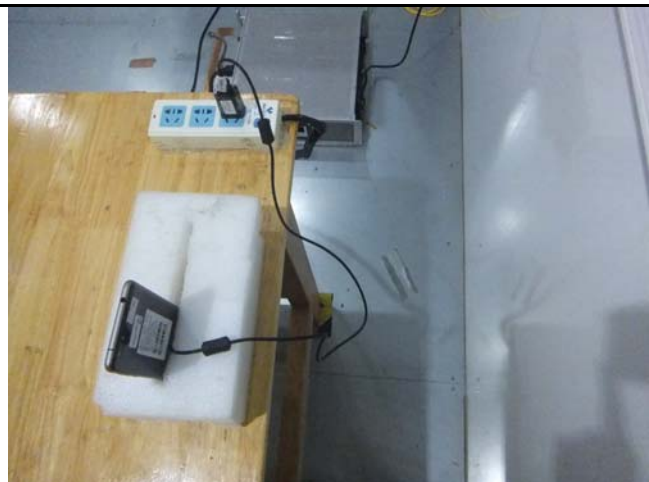
Conducted Emissions Test Setup Side View
