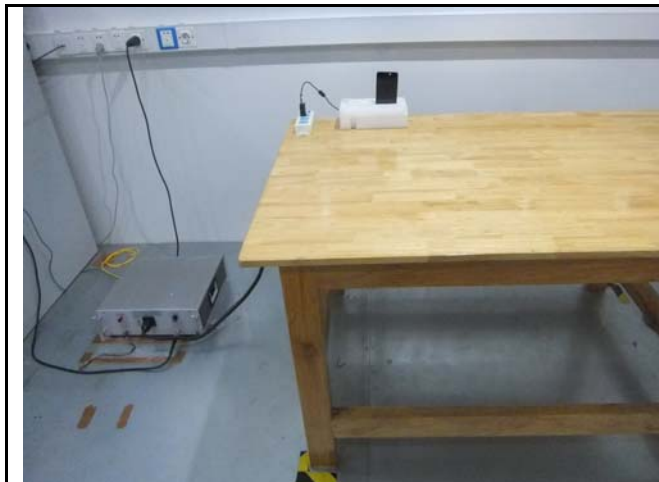
Conducted Emissions Test Setup Front View
