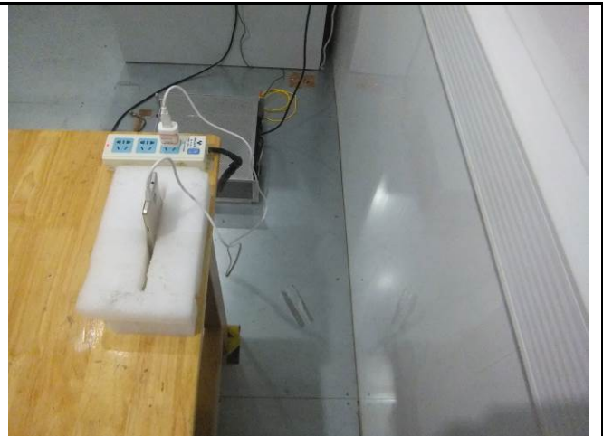
Conducted Emissions Test Setup Side View
