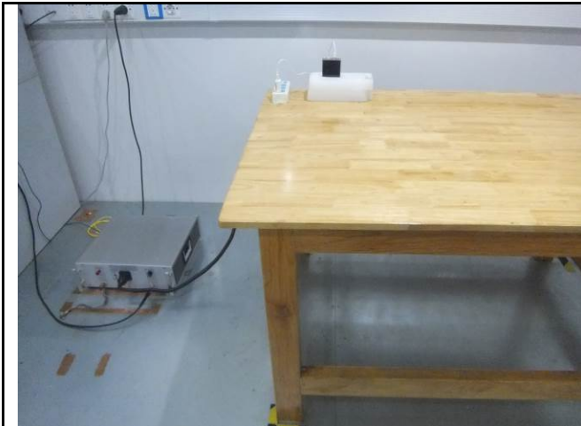
Conducted Emissions Test Setup Front View
