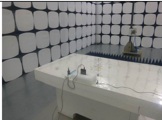
Radiated Spurious Emissions Test Setup Above 1GHz
