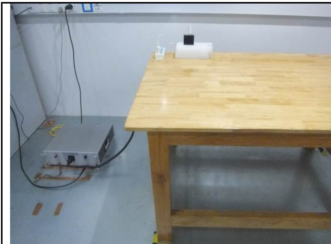
Conducted Emissions Test Setup Front View
