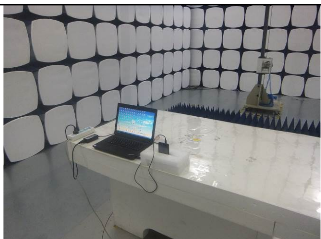
Radiated Spurious Emissions Test Setup Above 1GHz
