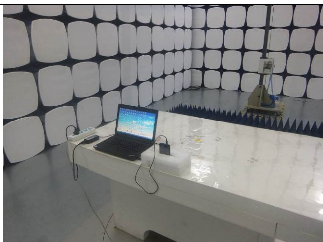
Radiated Spurious Emissions Test Setup Above 1GHz
