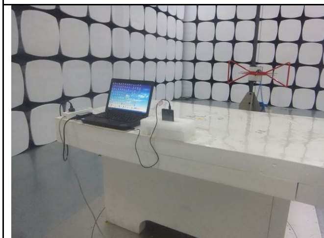
Conducted Emissions Test Setup – Front View
