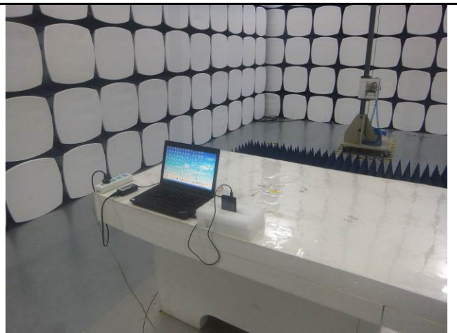
Radiated Spurious Emissions Test Setup Above 1GHz
