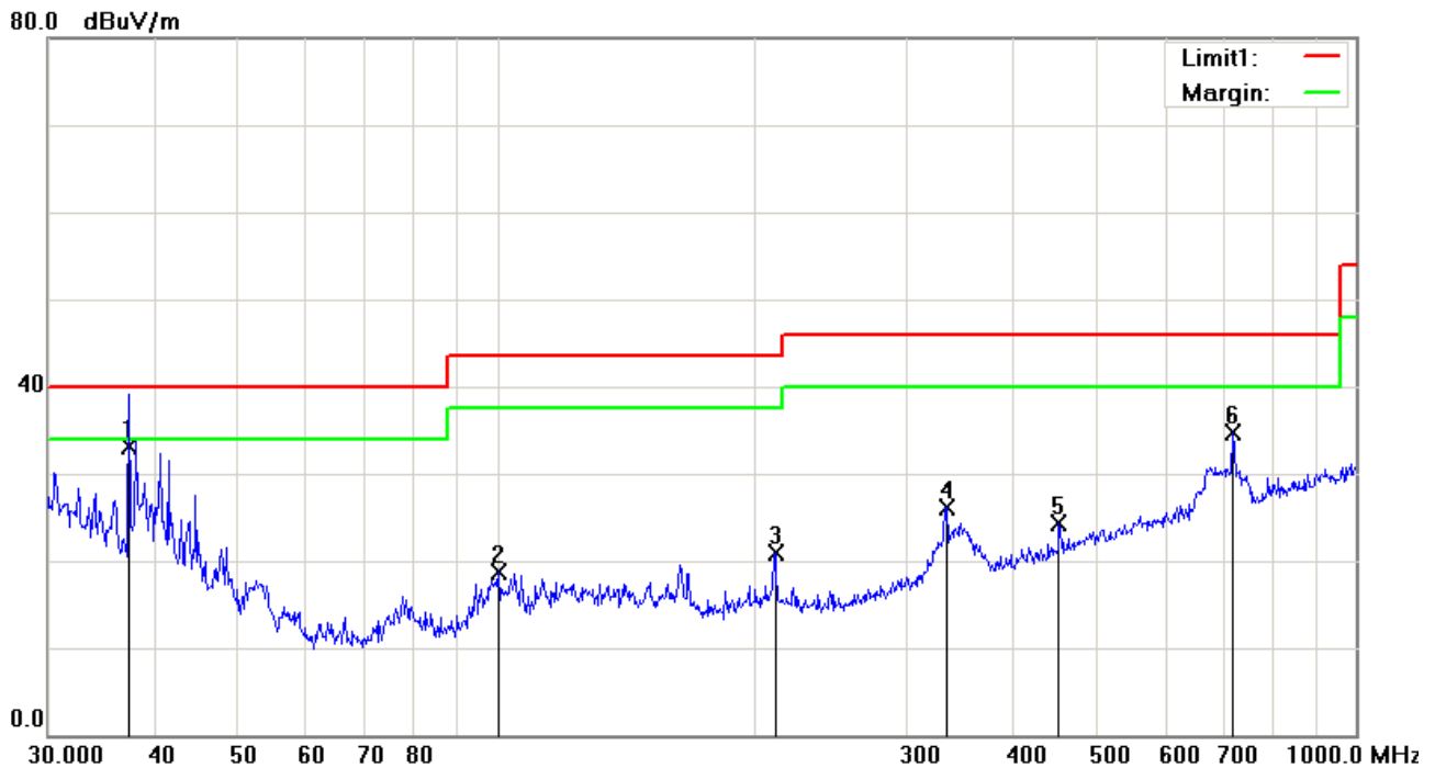
Horizontal Polarity Plot @3m
