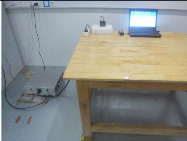
Conducted Emissions Test Setup – Front View
