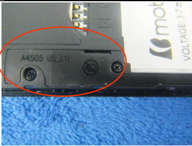
LTE- Antenna View
