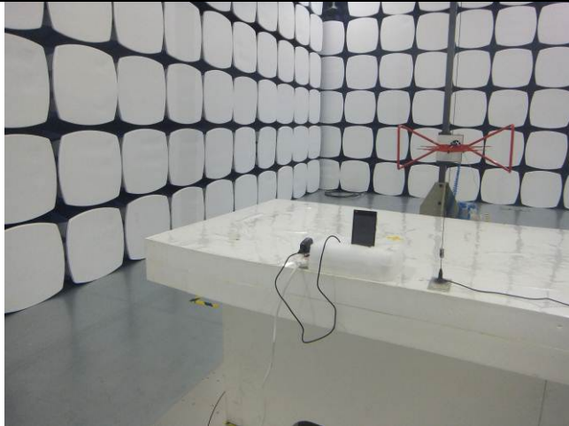
Radiated Spurious Emissions Test Setup Below 1GHz
